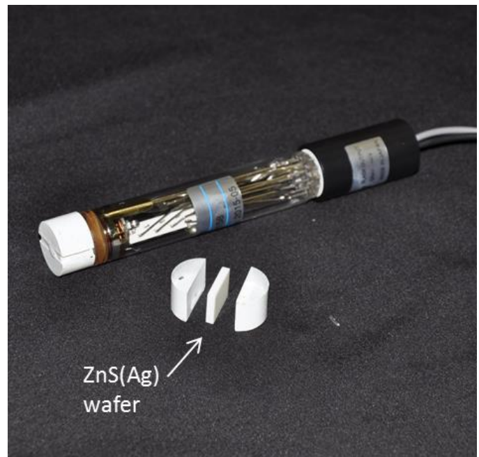
Fig. 1. A complete ZnS(Ag) detector assembly and a ZnS(Ag) wafer decoupled from the waveguides.
