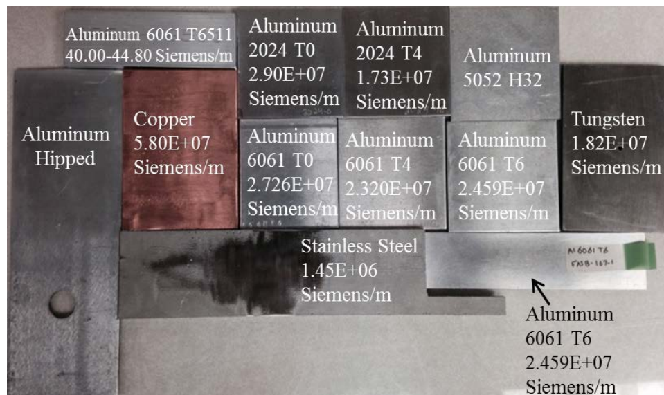
FIGURE 2. Materials with different conductivity values [3] affect the EC probe measurement.
