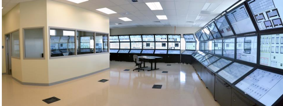
Figure 1: The Human System Simulation Laboratory (HSSL) with the generic pressurized water reactor control boards displayed on the three-screen bays.
