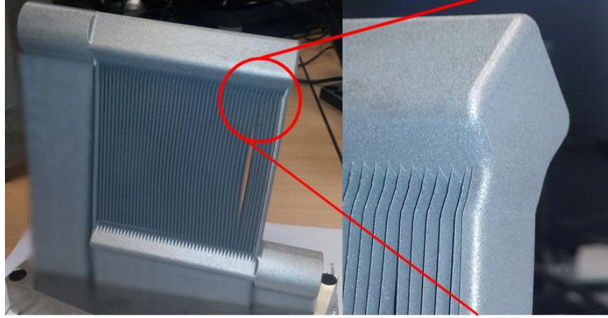
Figure 34 – 3D printed NURBS Shape Tube HX.
