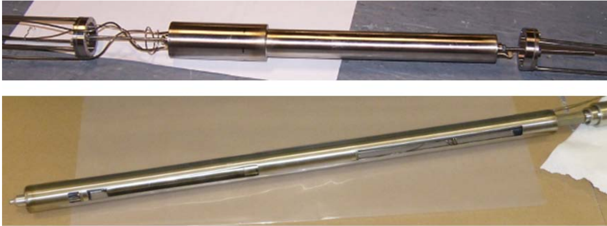
FIGURE 1. “Fuel rod” thermoacoustic sensor. (Above) The thermoacoustic resonator is shown at the center of the photograph. (Below) The resonator and suspension springs are contained within a “slotted tube” that has the same outer diameter as the reactor’s fuel rods. The thermoacoustic sensor can be designed to meet the same geometrical constraints as most fuel rods.
