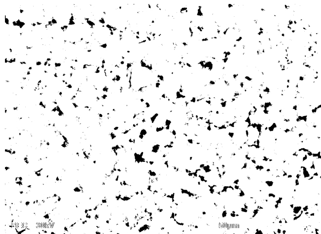
Fig. 5. BSE SEM image (500x magnification) of a TREAT LEU conversion compact after conversion to a binary – black and white – image by removal of the masked phases. The white portions of the image represent zirconia and graphitic phases. Non-graphitic phase are shown as black.
