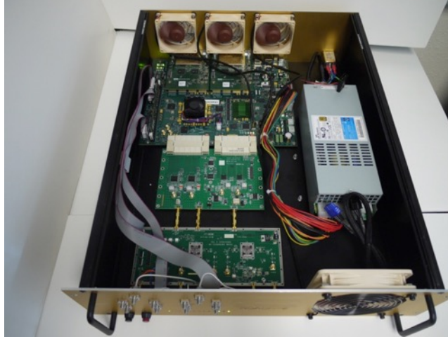
Figure 1. The ROACH2 (at back) in its new case with the ADC/DAC (middle) and IF (front) circuitry inside the case, improved cooling fans, front panel SMA connections, and a lower noise power supply. The pictured IF circuitry was later replaced with better performing custom IF circuits.
