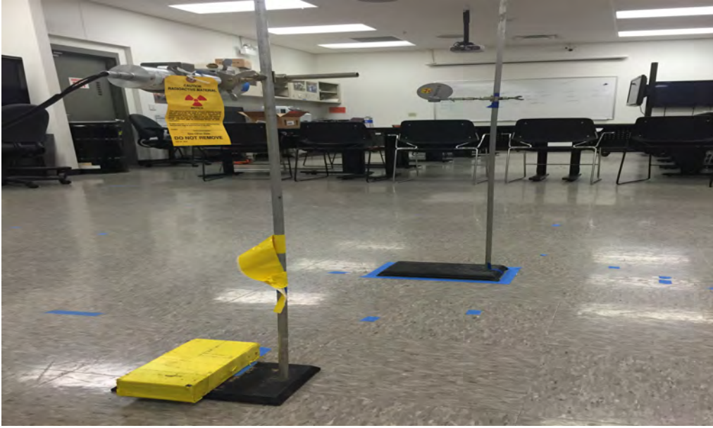
Figure 4.1 Photograph of the HEU Disk source measurement experimental setup.
