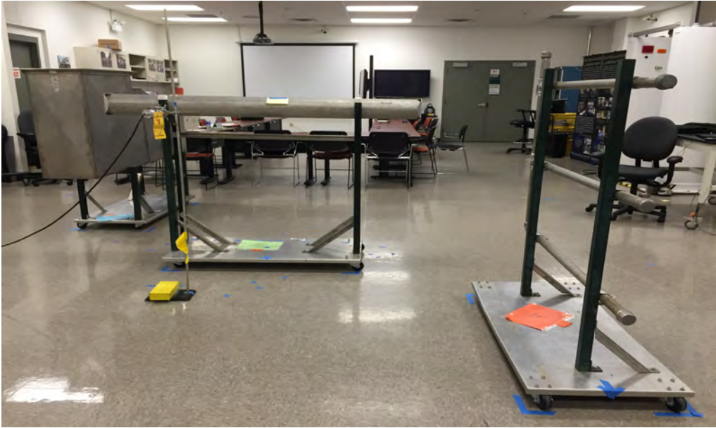
Figure 4.4 Photograph of the general holdup-like source measurement experimental setup.
