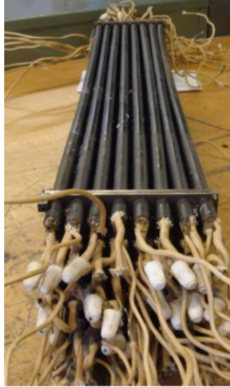
Figure 9: Square 8x8 array of heater rods, held by two spacer plates, removed from its pressure vessel. Heater power cables and thermocouple lead wires are seen in the foreground.
