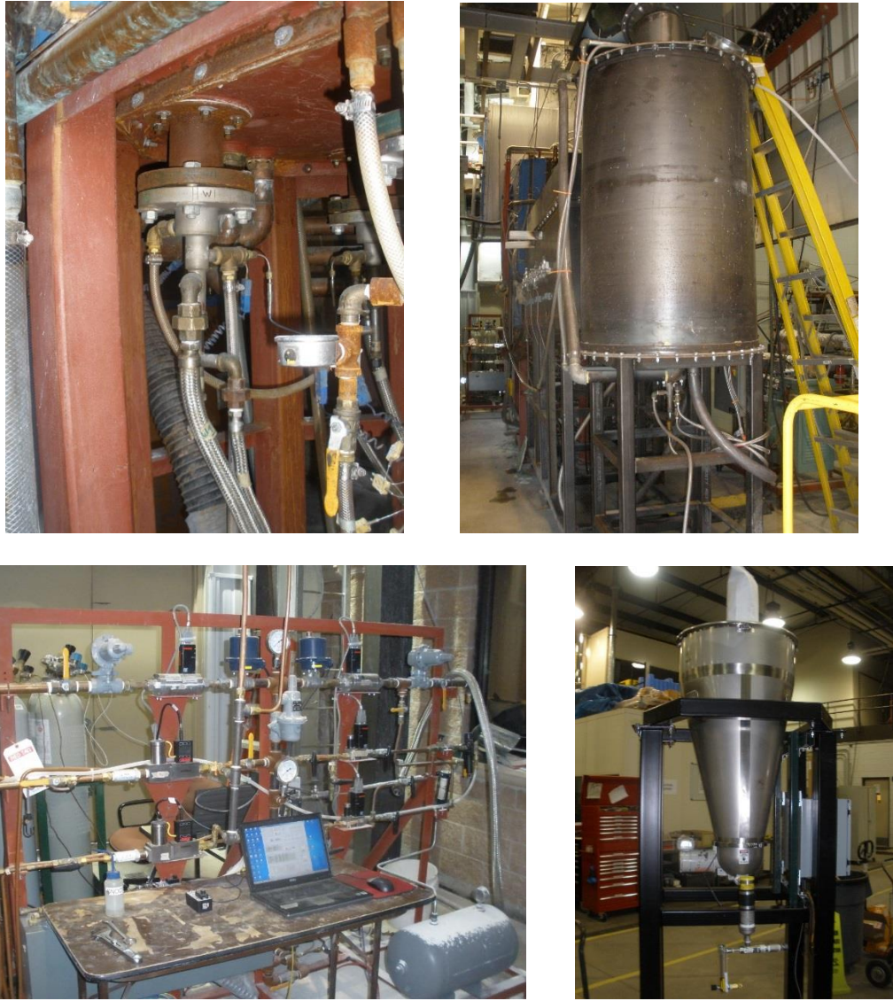
Figure 5. Photographs of the Oxy-Fuel Gas Burner, the HMB Gasification Test Unit, the Fuel Gas Blending Station, and the Coal Feeder
