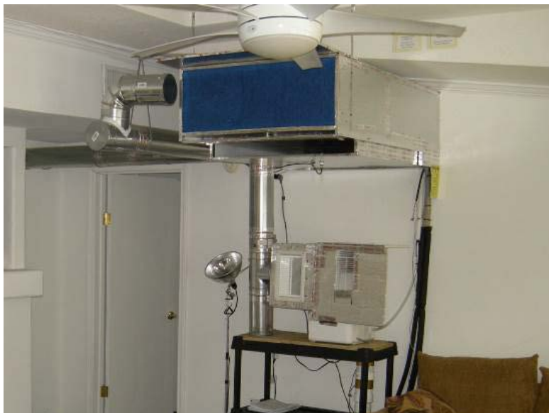
Figure 5. MSHP indoor unit mounted high on the wall in the MH Lab main space. The return air of the unit is enclosed in a plenum with a calibrated flow station. As shown, the OA duct terminates at the intake to the MSHP. It can also be directed to the dehumidifier unit below the MSHP or redirected further into the central space.
