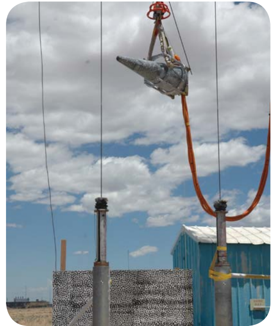
Sandia National Laboratories performs a drop test for the W88 Alt 370 program from its 185-foot Drop Tower Facility.
