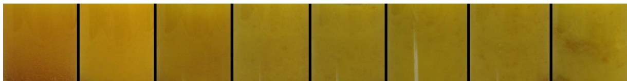
Fig. 6-9 Solution colors of 3 M MEA in DMSO with 1.5 g of \text{V}_2\text{O}_5 . Beginning from the left: 0 min, 5 min, 10 min, 15 min, 20 min, 25 min, 30 min, and 120 min, no reduction of \text{V}^{5+} to \text{V}^{3+} was observed in DMSO.
