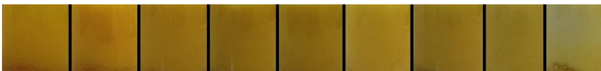
Fig. 6-10 Solution colors of 3 M MEA in MeOH with 1.5 g of V_2O_5 . Beginning from the left: 0 min, 5 min, 10 min, 15 min, 20 min, 25 min, 30 min, 60 min, and 120 min. Like in DMSO, there is no observable color change in the solution, aside from a slight discoloration at the end at 120 minutes, thus suggesting that there was no reduction of V^{5+} to V^{3+} .
