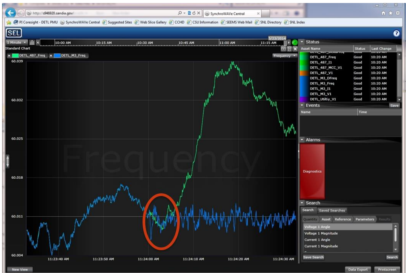
Figure 16. Screen shot of the local (blue) and remote (green) frequencies vs. time during one of the 4+ sec run-ons observed during Phase 1 testing.
