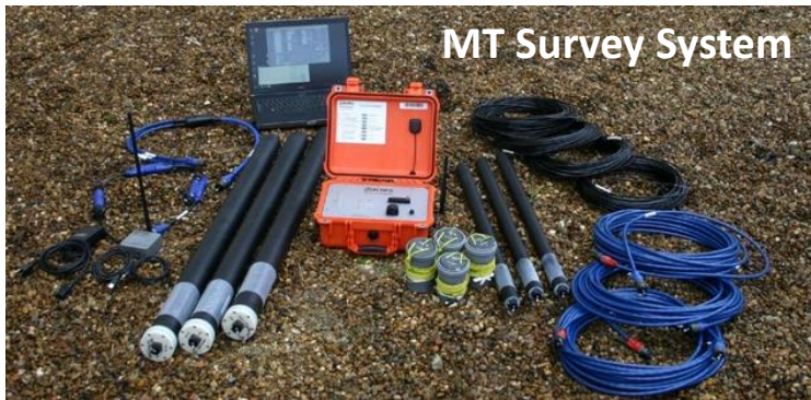
Figure 2. The field setup of an MT station with two electric field dipoles (Ex and Ey) and three orthogonal magnetic coils (Hx, Hy and Hz). The lower image shows MT equipment with magnetometer coils (black long cylinders) and four electrodes (gray and yellow).
