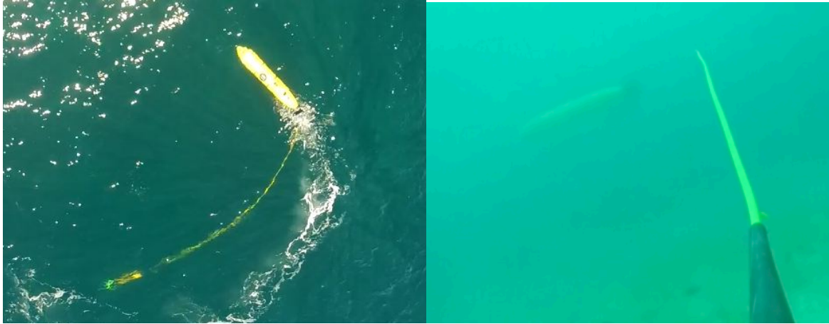
Fig. 12: AUV-towed magnetometer. (a) Aerial view, (b) View from the towed sensor
