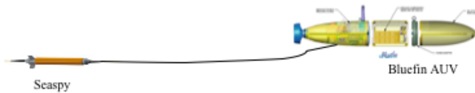
Fig. 2: Schematics of the towing of the SeaSPY magnetometer
