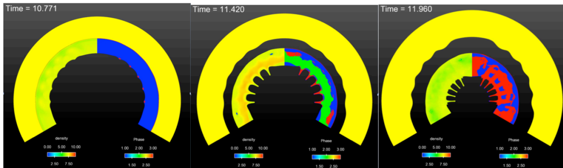
Figure 9. I = 0.8x , kA = 0.3 simulation. Spike release to liquid (red) but have their tips refreeze into the beta phase (blue) causing blunting at late time. The bulk transitions from beta to gamma (green) and liquid.
