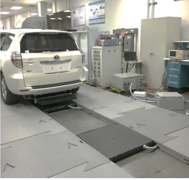
Fig. 3. Experimental Setup: A Two-Coil Track with Matched Coils
