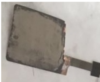
Figure I-26. SLMP coating on 12 cm 2 pouch cell with the optimized disperse agent, i.e.m 0.5 wt% SBR and 0.5 wt% PST in xylene solution.
