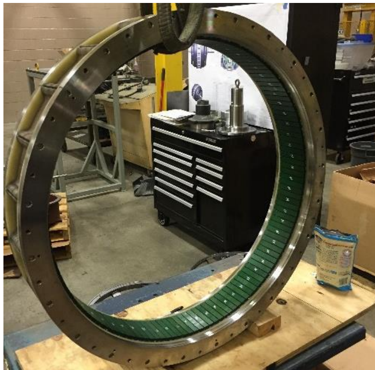
Figure 14. Low speed rotor with magnets installed
