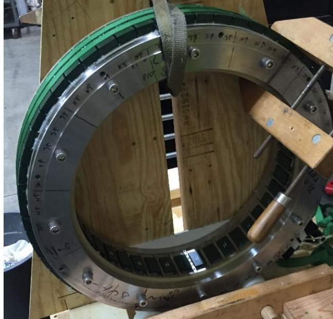
Figure 9. High speed rotor with wood clamp on last magnet until affixing epoxy set
