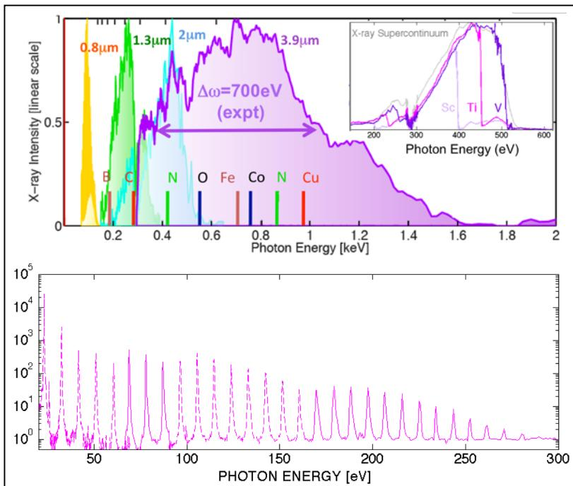
**Fig. 1. Bright high harmonic generation in near neutral gases (top) and multiply ionized plasmas (bottom).** (top) Bright coherent HHG X-ray super-continuum driven by mid-IR lasers, reaching photon energies  $> 1\text{keV}$ . The inset shows the first bright HHG in the water window at kHz rep rates, ideal as a backlight for probing WDM. (bottom) First bright HHG emission in plasmas ( $\text{Ar}^{5+}$ ). Bright UV-driven HHG extends up to 280eV, with narrow line widths ideal for imaging WDM.
