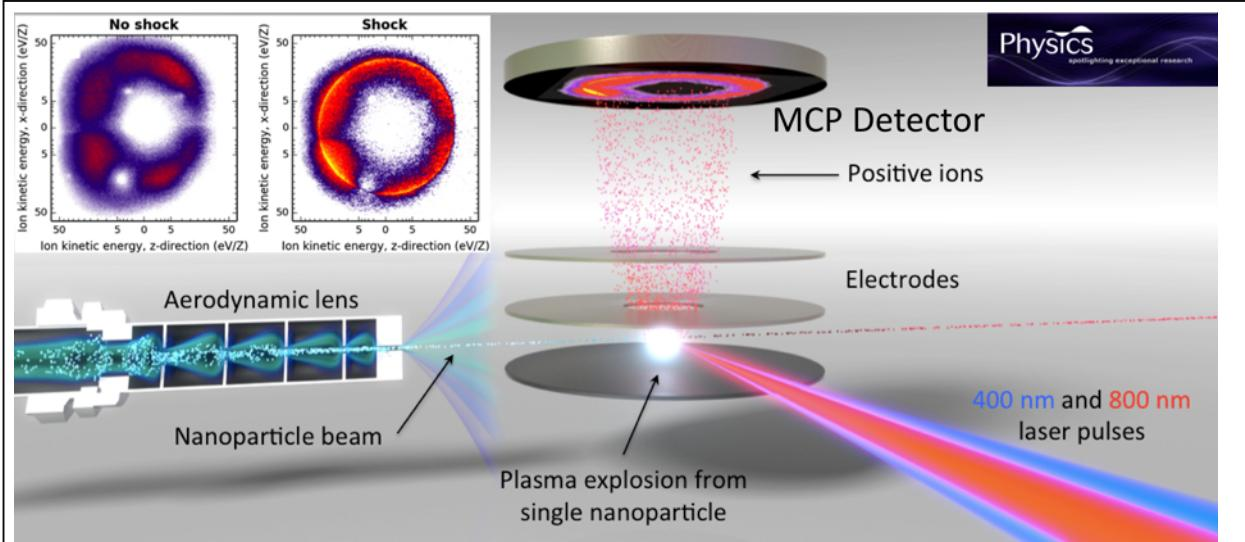
**Fig. 2: Imaging shocks in nanoplasmas.** An aerodynamic lens produces nanoparticles which are irradiated by one or two time-delayed laser pulses to generate an expanding nanoplasm. (left inset) The photoion angular distribution from a  $\text{NH}_4\text{NO}_3$  nanoparticle typically displays a broad ion distribution. However, if the particle size, laser intensity, and laser pulse time-delay are tuned appropriately, a sharp shock wave (yellow) appears.
