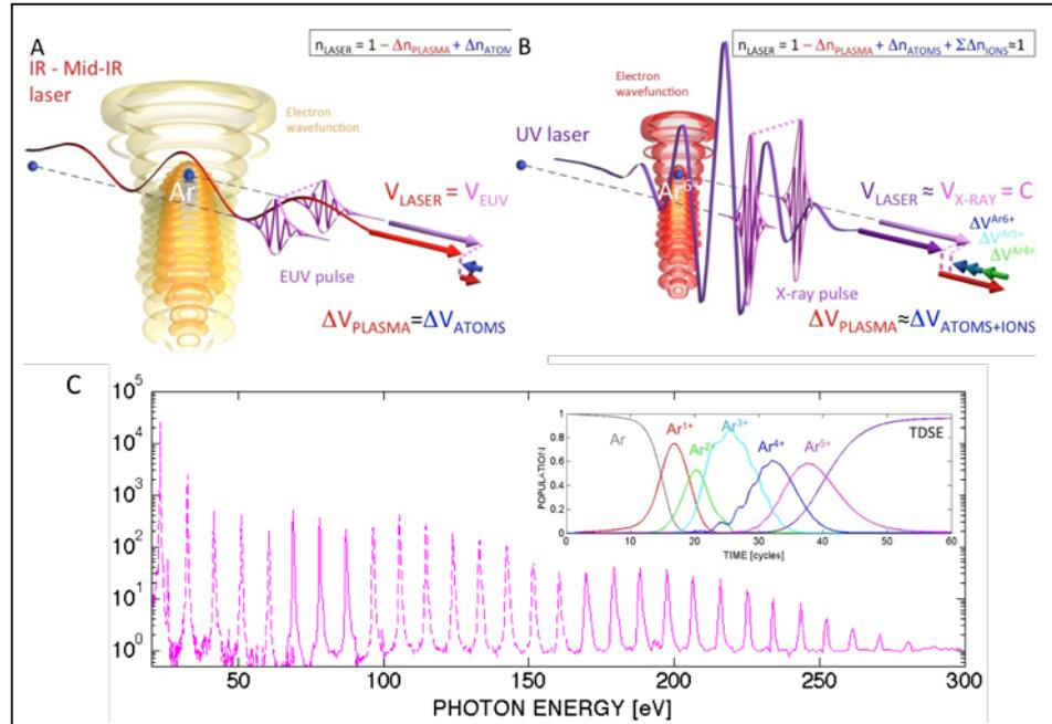
**Fig. 4. Phase-matched or near-phase matched HHG in highly-ionized plasmas.**
