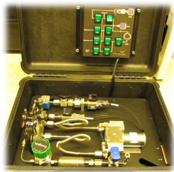
Figure 47. The calibration suitcase was developed to repeatedly and consistently deliver calibration gas to IMS stations.
