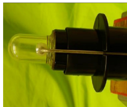
Figure 54. Example of a 4 cm 3 (~1 cm x 4 cm) plastic scintillator beta cell used in current \beta - \gamma detectors, designed to fit inside of a NaI detector well.
