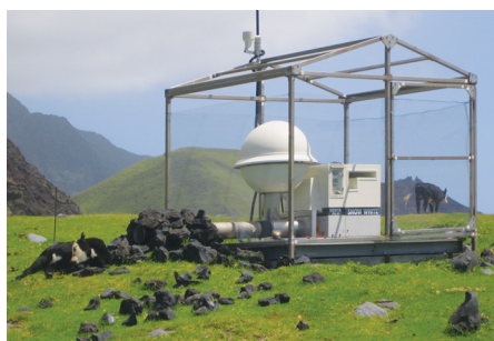
Figure 56. The Snow White air sampler as developed by Finland. Credit: CTBTO Preparatory Commission.
