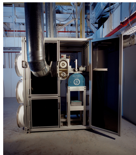
Figure 57. The RASA system as developed by the U.S., with a system footprint of 1m x 2m.
