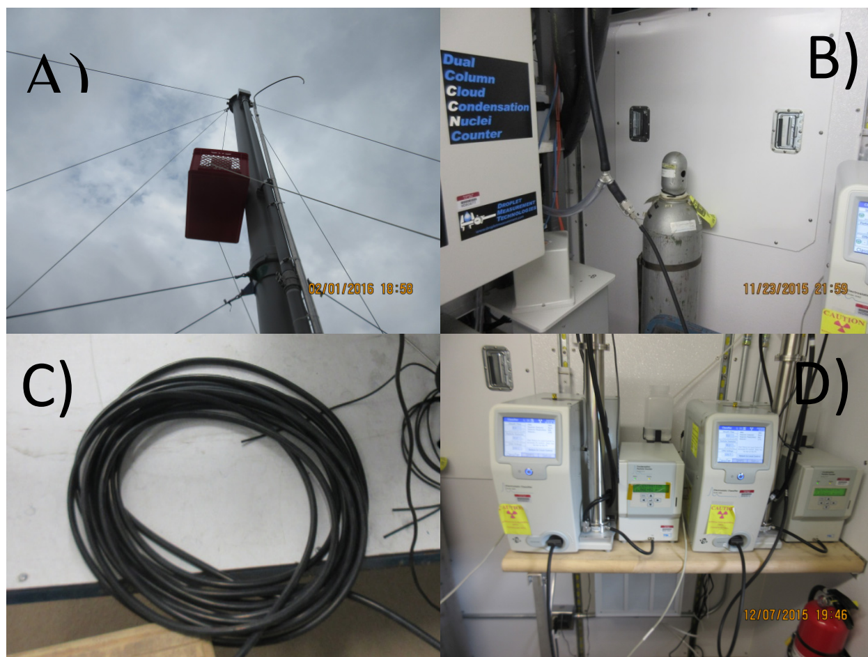
Figure 4. A) Line run to the top of the stack for the ambient measurement, complete with rain guard. B) Core inlet extractor from side flow distributor port (used for SMPS and UHSAS). C) Coils used in SMPS experiment. D) Side-by-side SMPS measurements.
