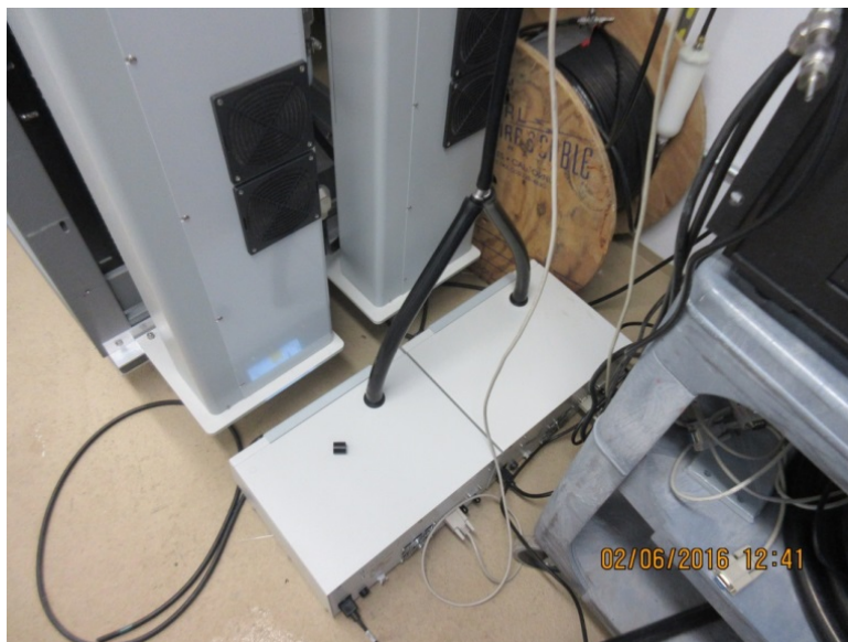
Figure 6. Side-by-side APS sampling for instrument bias correction.
