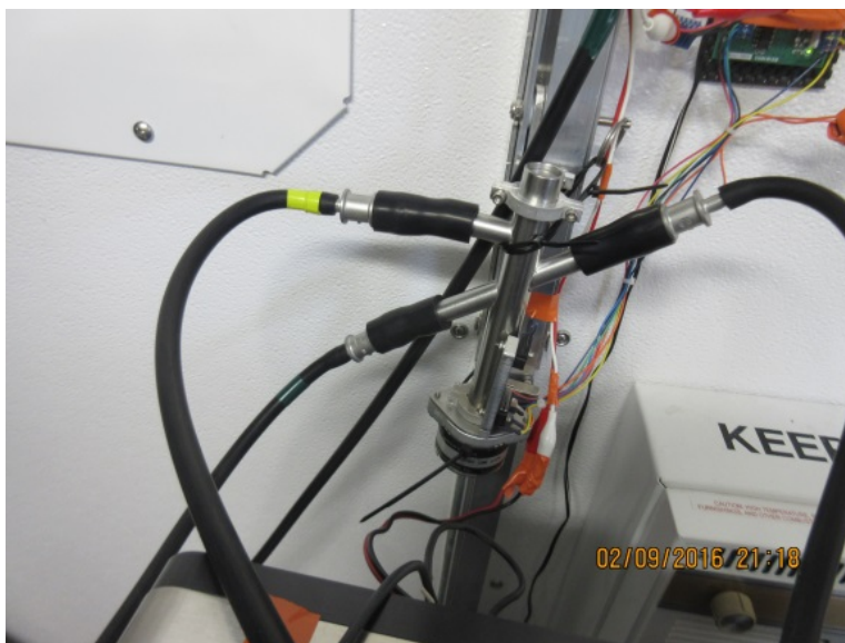
Figure 5. Fast-switching, three-way valve used for the UHSAS portion of inlet characterization.
