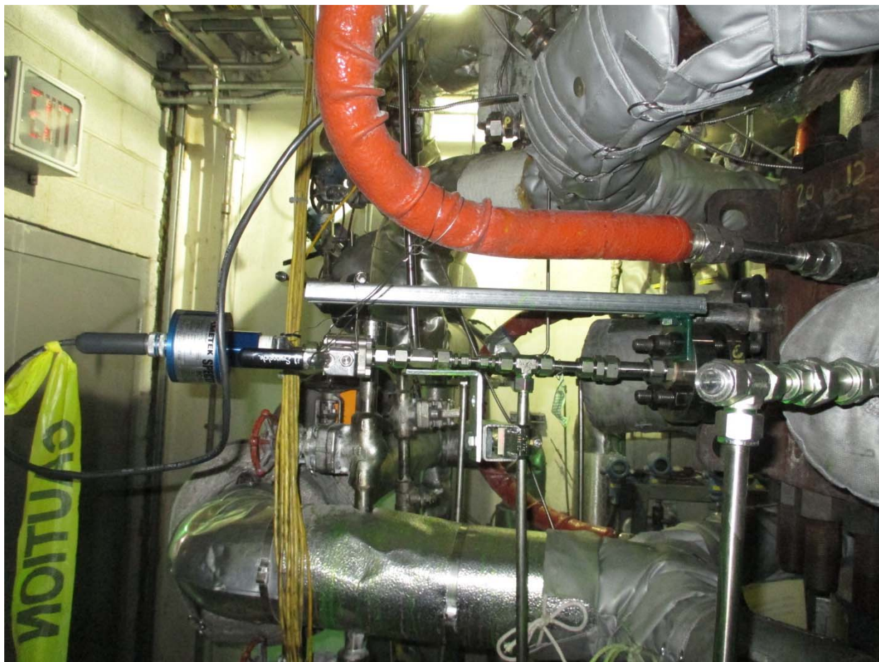
Figure 13. Wall wash lance design with integral view port passageway installed at gasifier outlet, in the same plane as the quench lances.
