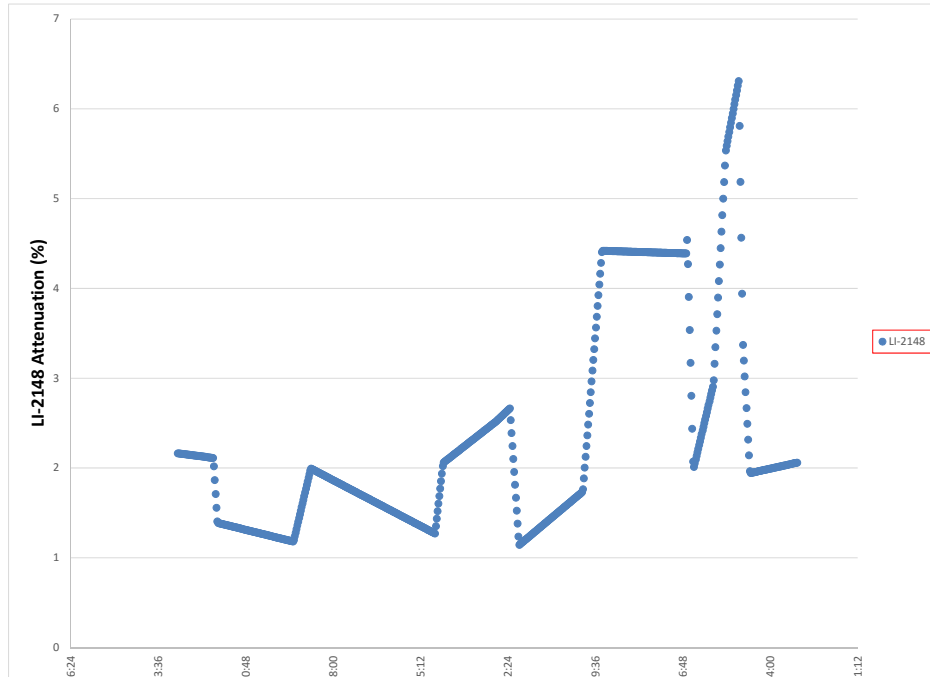
Figure 9. Example of results from LI-2148 Vega Americas detector for indication of solids build-up in quench vessel during testing. Data in the figure are from test operations, showing both accumulation of solids as well as removal of solids using the wall wash quench lances.
