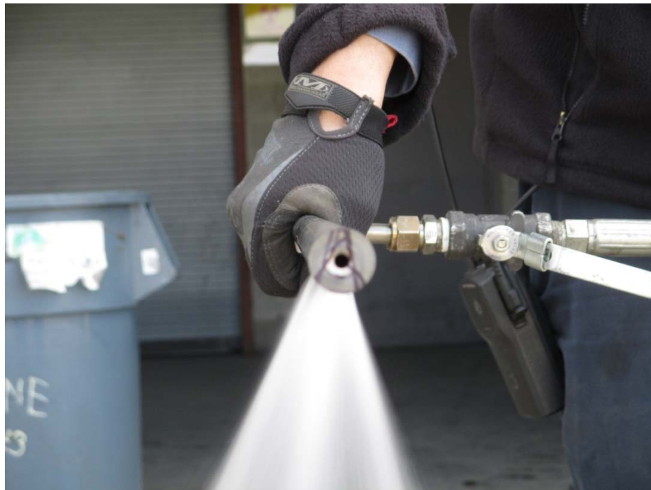
Figure 12. Atmospheric testing of the wall wash lance was used to evaluate spray pattern and to assess flow rate as a function of pressure drop.
