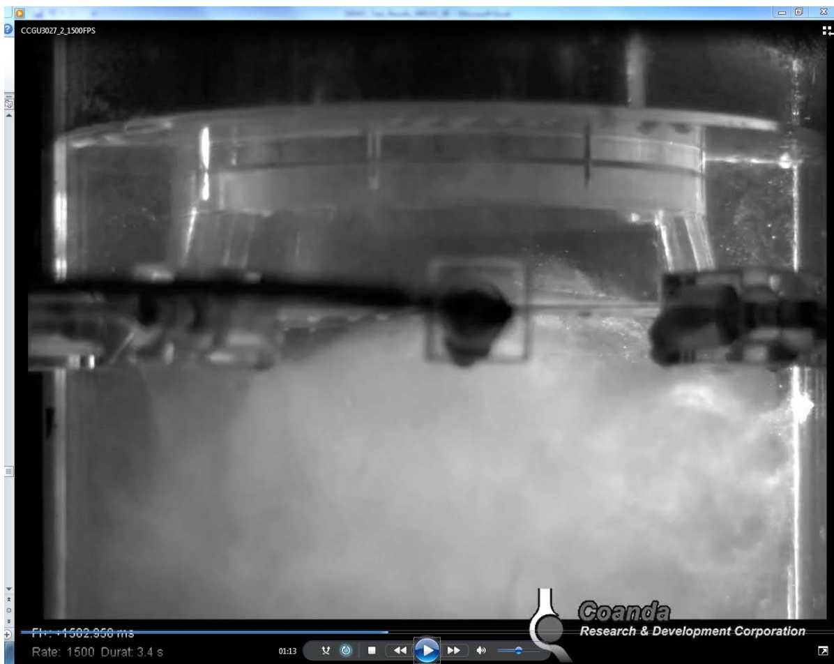
Figure 17: View of recirculation into short outlet cone from Test 3027.
