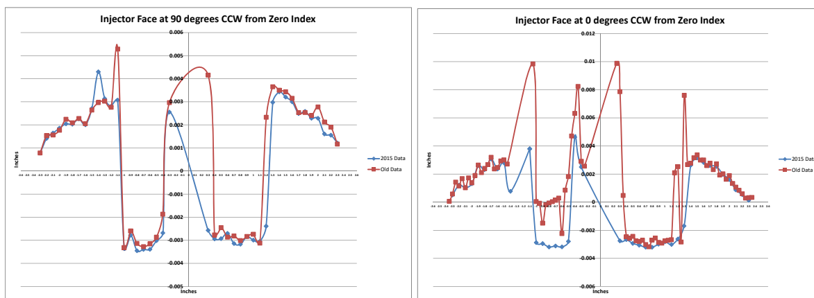
Figure 19. Profilometer traverses of the injector faceplate, showing loss of ~ 0.005" erosion resistant layer but no loss of parent material.
