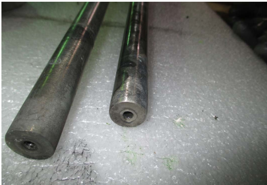
Figure 11. View of wall wash lance with integral view port, from the end installed in the gasifier. View port is via \frac{1}{4} " tube in the center. Wall wash spray is via the horizontal slit in the \frac{3}{4} " tube wall located about 2" from the end of the lance.
