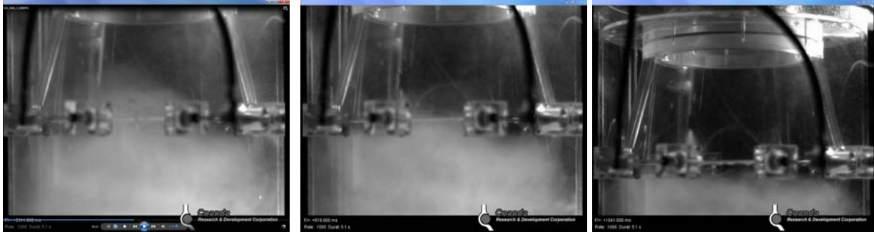
Figure 20: Impact of decreasing liquid/gas momentum ratio on quench spray intrusion into cone. Momentum ratios of 2.24 (left, Test 3036), 1.35 (center, Test 3037) and 0.84 (right, Test 3038).
