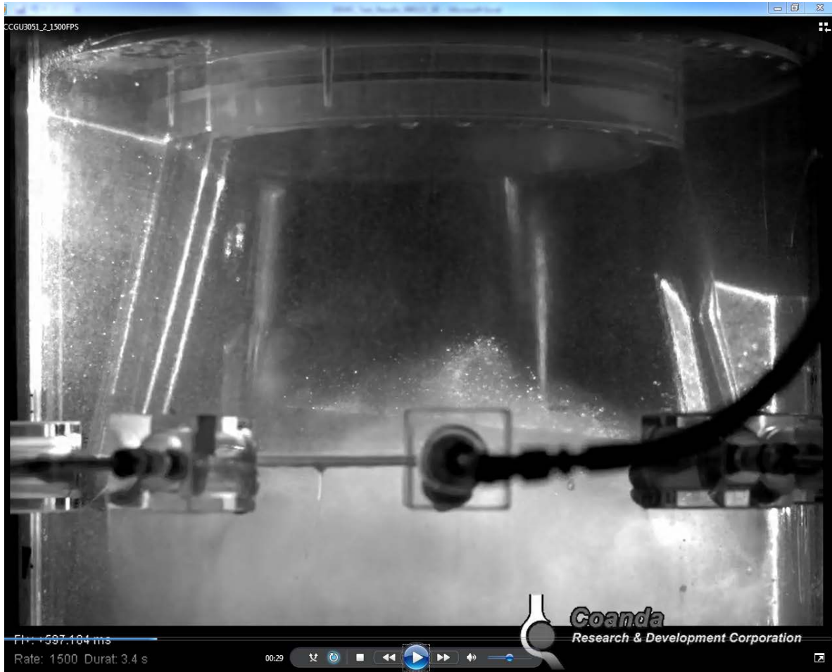
Figure 18: View of recirculation into baseline (long) outlet cone from Test 3051.
