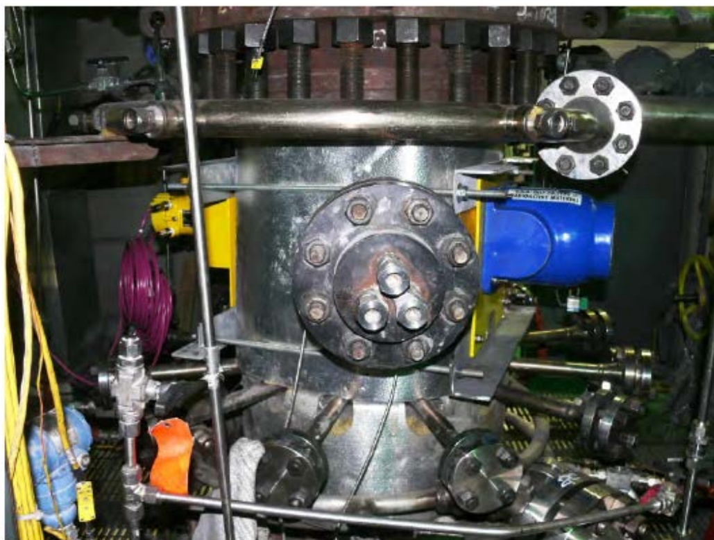
Figure 15. View of gasifier quench vessel just downstream of gasifier outlet, showing installation of Vega Americas gamma source (blue device on the right) and MiniTrac detector (yellow device on the left). This system provided real-time detection of solids build-up within the quench vessel.
