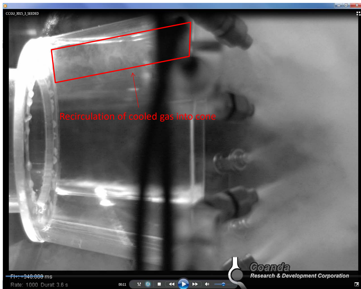
Figure 14: Testing with HA134a as quench liquid in Test 3015, using gas seeded with water vapor to highlight flow patterns of cooled gas. The water vapor condenses/freezes upon contact with HA134a, creating a cloudy gas roughly analogous to quenched syngas.
