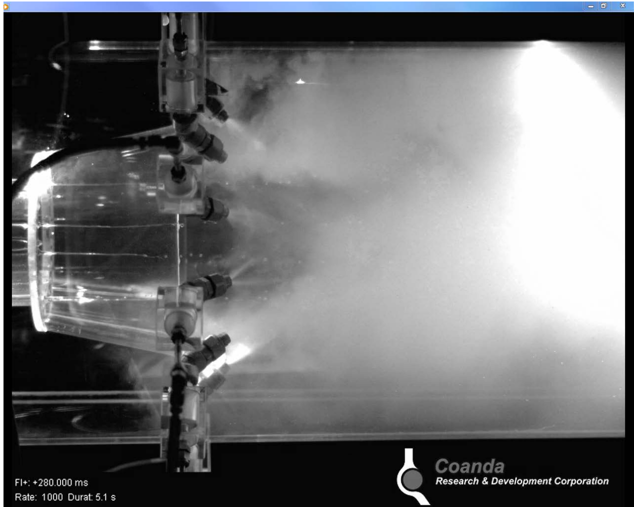
Figure 15: Testing with HA134a as quench liquid in Test 3016, with simulated slag flow.
