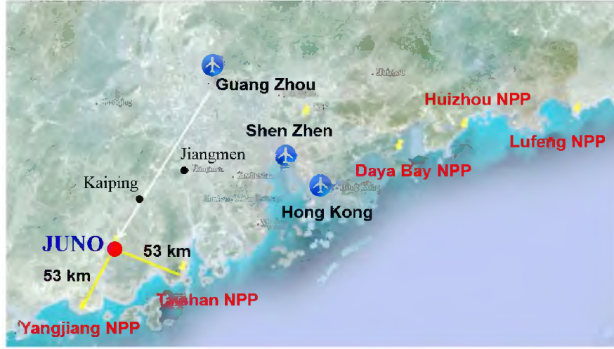
Figure 1-3: Location of the JUNO site. The distances to the nearby Yangjiang NPP and Taishan NPP are both 53 km. Daya Bay NPP is 215 km away. Huizhou and Lufeng NPPs have not been approved yet. Three metropolises, Hong Kong, Shenzhen, and Guangzhou, are also shown.
