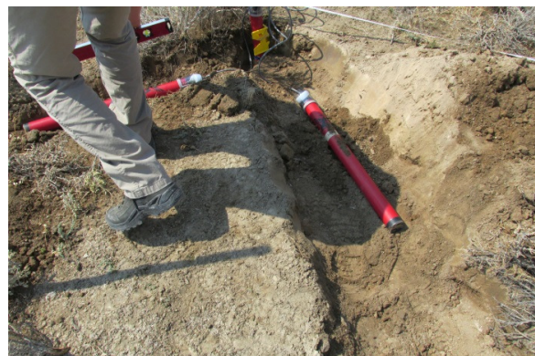
Figure 5. Set up of the single direction magnetometer coils.
