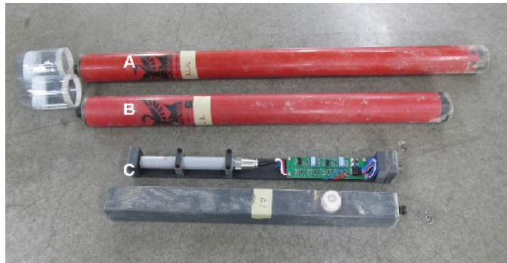
Figure 6. The Phoenix Geophysics A) Low Frequency mag B) High Frequency mag and C) MPT three-flux gate magnetometer.
