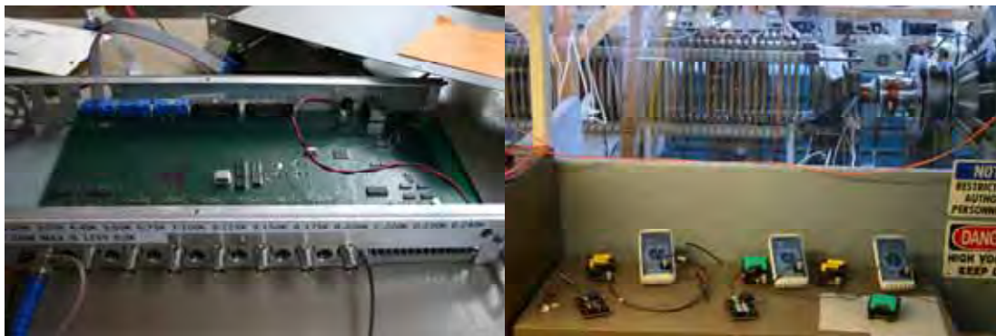
Figure 4.16.1.1. Bank voltage remote control systems. (left) The first prototype 8 channel microcontroller with Ethernet control system. The BNCs and IDCs are for manual monitoring and set points during the test/verification phases. This system can be compacted to a CAMAC slot profile once the design is verified. The system is currently set for manual input (as a bank of 8) with the set voltages being controlled by one dial (via an IDC connector at rear). Interlock connectivity is also accomplished via a rear IDC port. Ethernet hardware functionality has been tested but the final routines to implement an interrupt driven system have not completed testing for lack of time. DIP switches allow for changing the counter clock base in powers of 2. The prototypes are used to control the reversal and bias banks. At least one IDC port will be retained to allow for microcontroller programming in system and features not yet considered. The interlock fiber transmitter/receiver may be integrated into the final board. (right) Three channels of pure manual control. One unit converts the fiber frequency to BNC. The meter displays the frequency. A second unit generates the three state bank control signal. It is expected that even upon completion of the automated system these units will be used for testing/troubleshooting purposes. The three state bank control unit is also useful for test firing (because the momentary charge button is de-bounced).
