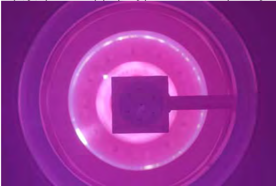
Figure 4.14.2.8. Copper capped MPD blocked by SXR diagnostic on east end of experiment. The SXR diagnostic design was looking forward to a time when the MPD sources would no longer be on axis. Unfortunately, this early test of the diagnostic had no definitive results. The ratios of the different x-ray spectra did not give self consistent results for derivation of temperature. One might speculate that this could be due to unanticipated plasma contaminants.
