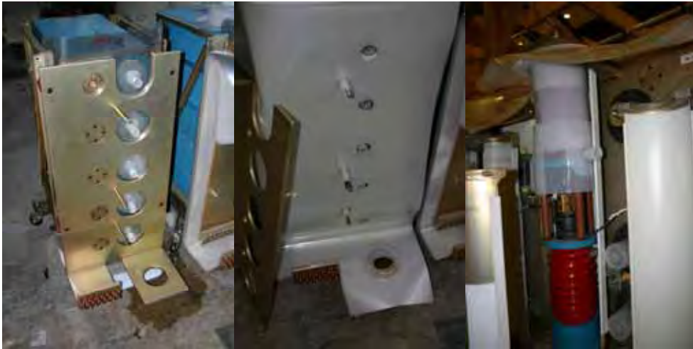
Figure 4.4.1. LSX reversal bank module design. This picture shows one half (-) of a pair (+/-) required. Various states of assembly are shown. The final assembled state (not shown) has two conductive feeds (half cylinders) around the ignitrons. Suspicion has arisen that the current feeds are sufficiently asymmetrical as to preferentially form the current channel in the switches off to one side.
