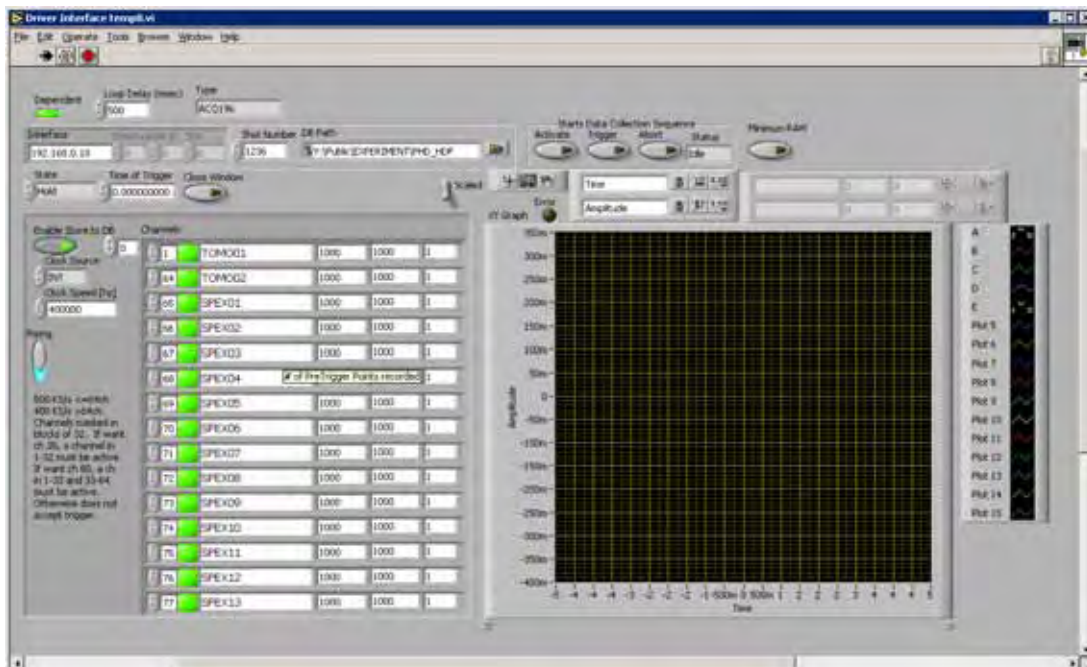
Figure 3.11.2.4. D-TACQ Solutions ACQ196 Series. \leq 96 channel, 16 bit, \leq 500 KHz, \leq 1 GB RAM total, Transient (or continuous with driver modifications) digitizer. Ethernet interface. Note that this hardware requires significant set up accomplished outside Labview.
