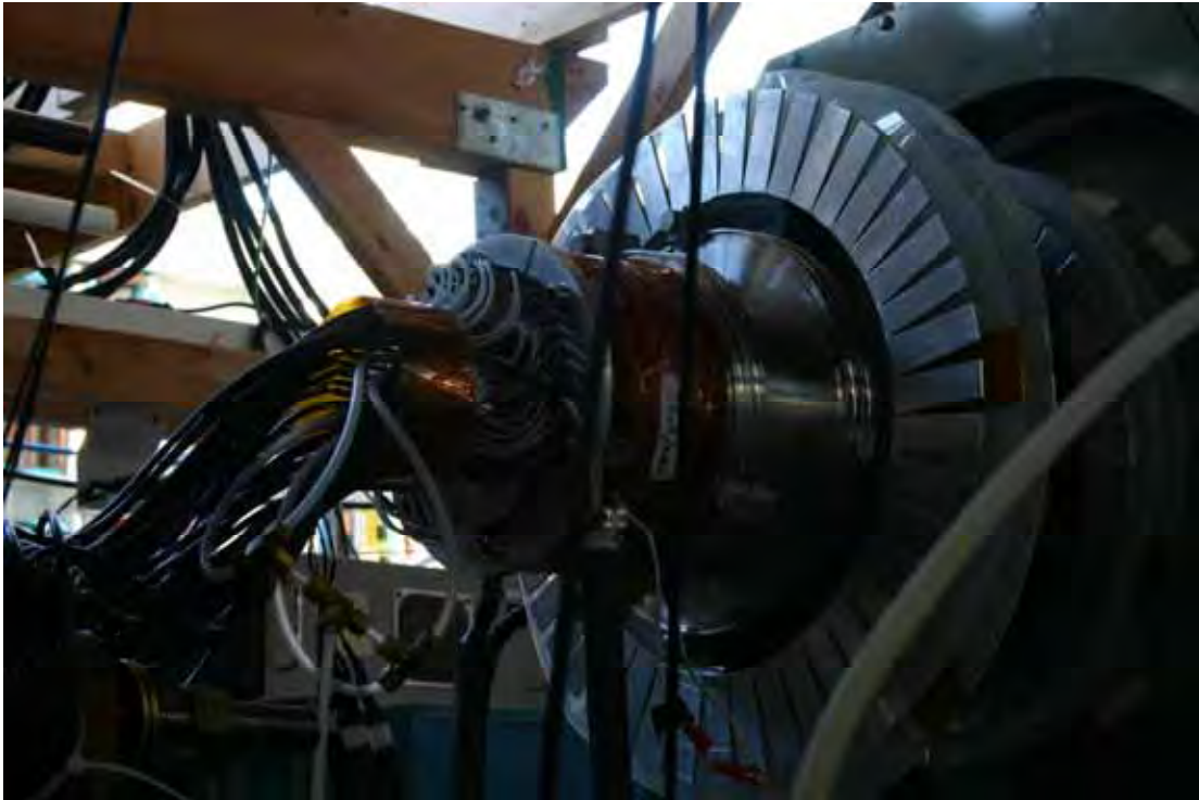
Figure 4.14.2.2. MPD hardware in place on +z end of machine. The original magnetic field coils are also clearly visible. Only one cathode rod's voltage is measured through a resistor and current pick up loop. The MPD current measurement is inferred from the sum of several individual cathodes.
