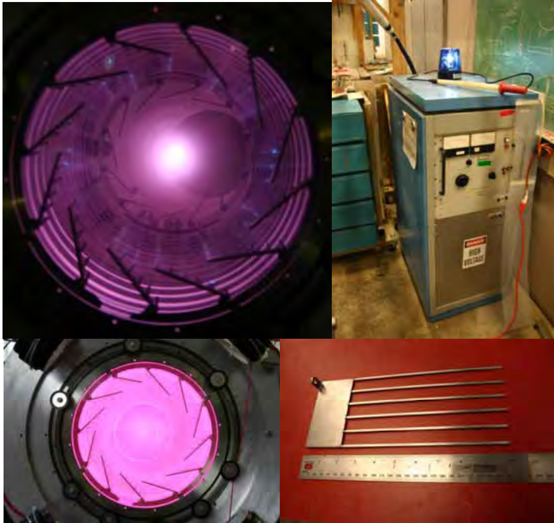
Figure 4.12.1. Axial discharge arrangement on 40 cm experiment. (top-left) The radially compressed non-ringing PPI can be easily seen. (top-right) The PPI bank was inherited from LSX. (bottom-left) The SPI lights up the whole tube. (bottom-right) Highly distributed stainless steel electrodes help to result in an azimuthally even discharge.
