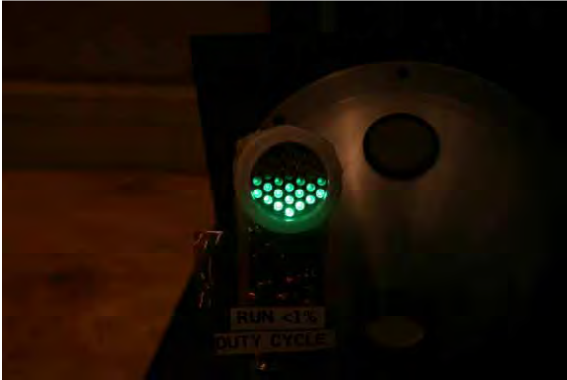
Figure 5.8.3. Not all pixels are acquired at the same time. The green LEDs are all on at the same times. It is presumed that near the beginning and end of capture not all the camera's pixels are acquiring, resulting in this very rare shot (exposure time: 1/60^{\text{th}} sec).
