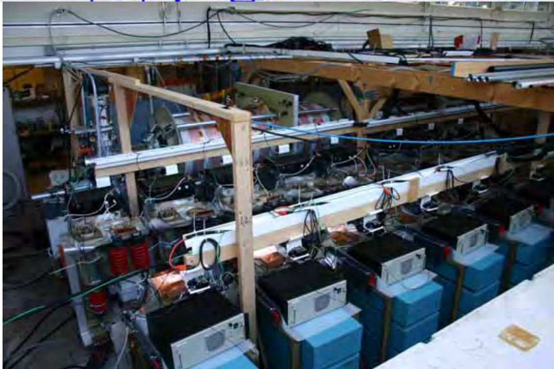
Figure 3.0.1. Experimental layout. This image was taken from a position near the plug bank. At this stage of the experiment, the standard turbo pump has been replaced with a magnetically levitated turbo. The magnetically levitated turbo is not adversely affected by the experiment due to the short duration of the experimental axial fields and the heavy metal walls of the turbo.
