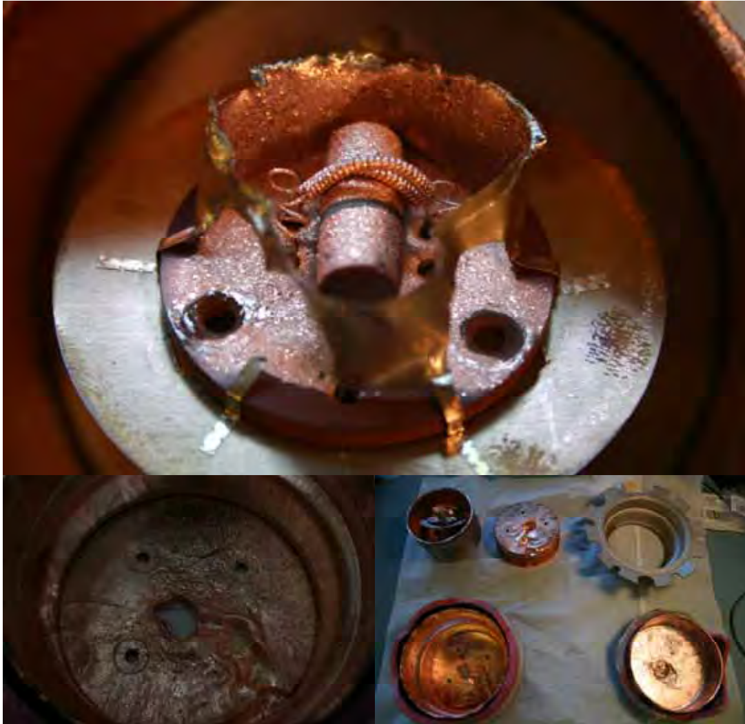
Figure 4.7.2. Pseudospark switch tested to destruction. The unit had switched a total of approximately 15 MJ in a ringing application over its lifetime. A switch in a crowbar position lasted roughly 24 kC at just over 4 coulombs per shot. The center hole (lower left) did not originally exist. A copper electrode eventually eroded away resulting in the coating of the trigger semiconductor with copper. The hydrogen reservoir is hidden beneath the plate holding the trigger. The obvious mechanical damage was incurred while breaking open the ceramic switch. Our ignitron trigger units were readily adapted to drive these switches even to this level of copper coating. We do not believe this level of coating was accomplished in just one shot. In applications without perfectly symmetric current feeds (i.e. in a mod) we've seen similar switches come up to air via a hole punched in the electrode corner.
