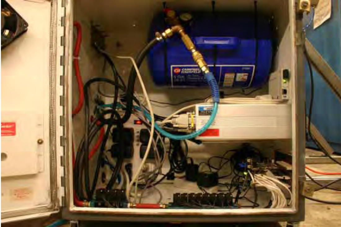
Figure 3.7.1. Vacuum control electrical enclosure. An air pressure reservoir can be seen at upper right along with the vacuum gauge controller (middle right) and air pressure actuator valves (bottom) driven by a microcontroller control board (lower right).
