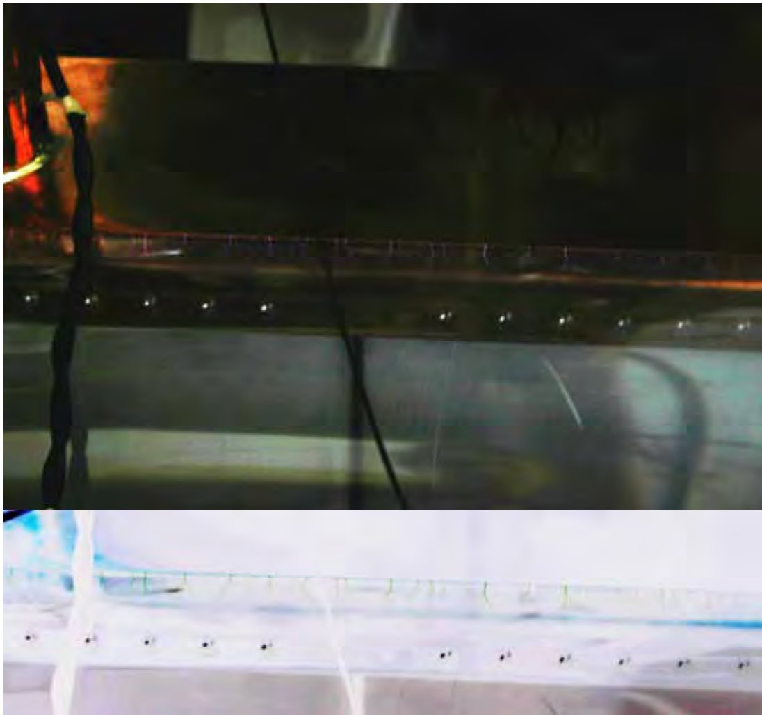
Figure 4.2.2. This is an example of corona caused by an edge and thin insulation. The capacitors are rated to 30 kV. A cropped negative is shown below the original image. The crackling of static electricity moving around could be heard leading us to take this exposure.
