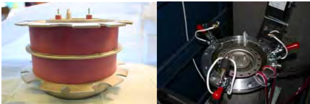
Figure 4.7.1. Pseudospark switch pictures. The devices are permanently sealed and easily mounted on Syllac header capacitors for use in oil. The installation at right is a Diala AX oil immersed switch test / conditioning fixture.
