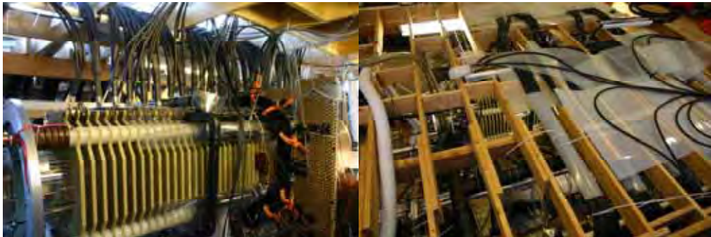
Figure 4.11.1. 40 cm experiment axial field coil layout. (left) One bias module \pm pair was used to drive the three coils at left in series, parallel with the opposite end (smaller diameter coax). This formed a cusp with respect to the bias field in the center section (small diameter coax). Two bias module \pm pairs are used to drive the center section coils. The central coils are driven with 2 coils in series, all the sets in parallel due to the bias connections.
