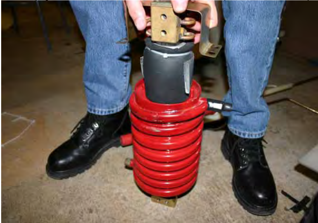
Figure 4.6.1. EEV BK488D type D ignitron with thermally insulated glass envelope. Flexible metal connections must be used (typically on anode) to prevent the build-up of mechanical stress in the device. Here, a thin metal strap is used to make the electrical connection. The painted red metal cooling jacket is the most apparent feature of this model of ignitron.
