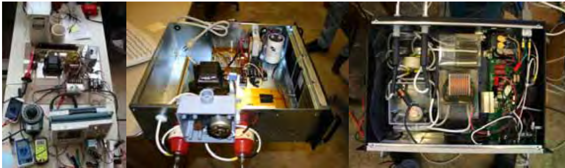
Figure 4.4.5. New HV power supplies from the prototype stage to production. Note that the final unit includes a dump relay and floating voltage outputs. The dump relay in this model is capable of reliable operation up to about 30 kV after which the generated corona causes sporadic contained arcs (non-damaging). A replacement relay has been made and tested but is not as cheaply produced as the original. The final unit has not yet been fully optimized. This picture is not representative of the final design. It represents a limited production model put in place due to time constraints.
