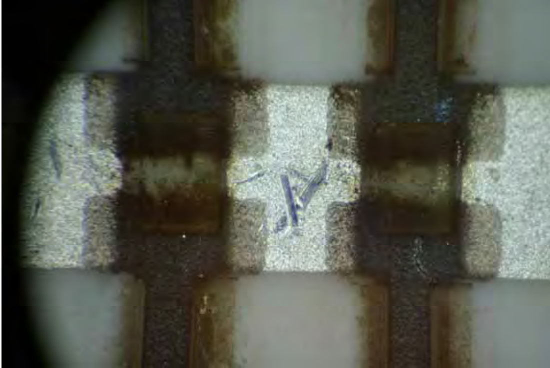
Figure 5.12.1. Damaged 5x coaxial BNC attenuator (2W). A crack due to excessive power input (100 volt levels, pulsed RMF monitoring) is visible in the lower right corner. Centers feed in on left and right. Outer ground shell attaches top and bottom.
