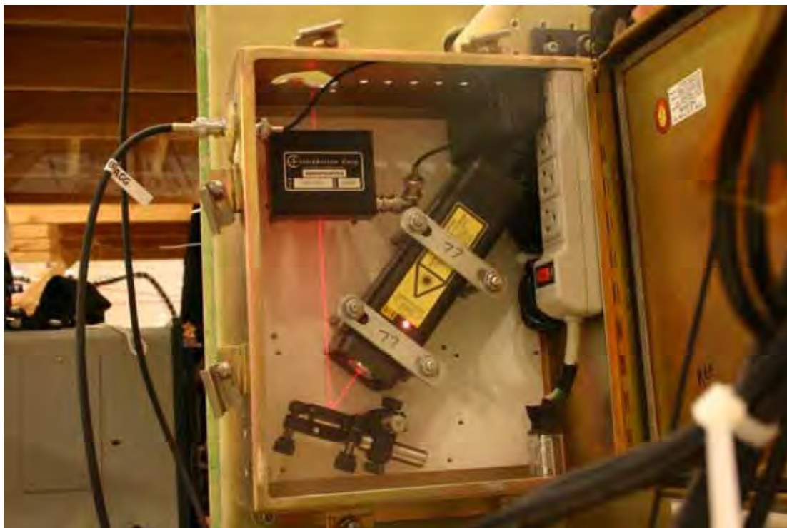
Figure 5.2.1.2. Bragg cell and laser enclosure. As can be seen, the Bragg cell (upper left corner) is kept electrically isolated from the rest of the box. The Bragg cell is an IntraAction AOM-402AF1. The laser source is a JDS Uniphase 4 mW HeNe laser. The laser is less than 16 cm long. The overall metal enclosure dimensions are 25 x 30 x 13 cm.
