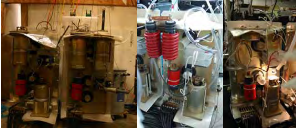
Figure 4.4.2. Module evolution. (left) The first modification made upon receipt of the old LSX modules was to add wheels to make it possible to move without a ‘walky stacker’. This was rapidly followed by changing the ignitron stacks to singles in order to reduce stray inductance (and provide spare ignitrons). The output cables were also changed from a sliding banana plug connection to a center screwed connection (where the screw carries little to no current). The ignitron igniters were made local to the module, soon to be followed by power supplies and dump capabilities. For testing purposes, our ad-hoc pole-transformer supply was capable of supplying kilowatts. The ignitrons could be rapidly heated. (center) The ignitrons were still undesirably inductive as start switches. To alleviate this problem, two are placed in parallel with their cooling jackets used as the current returns. Note that some of the crowbars have stainless steel current feeds (used as resistors). These resistors would frequently arc to the screw heads and other close metal surfaces during firing. These arcs would sporadically destroy and disconnect the resistors from the ignitrons throughout the experimental runs. (right) The start ignitrons have been replaced by copper vapor switches. The crowbars carry too many coulombs for a similar substitution to be advisable. A 50 watt halogen spot light shining onto a blackened plate connected to the crowbar ignitron’s anode can be seen; this provides a 30 C° temperature difference across the switch. Cooling of the cathode is still a potentially problematic issue given our region’s summer climate. Tests on the first module (left) suggested that when the cathode reaches the region of 30 – 35 °C very little voltage hold-off capability remains. Since we need to run ~ 30 switches reliably we need to keep the cathode temperature much lower.
