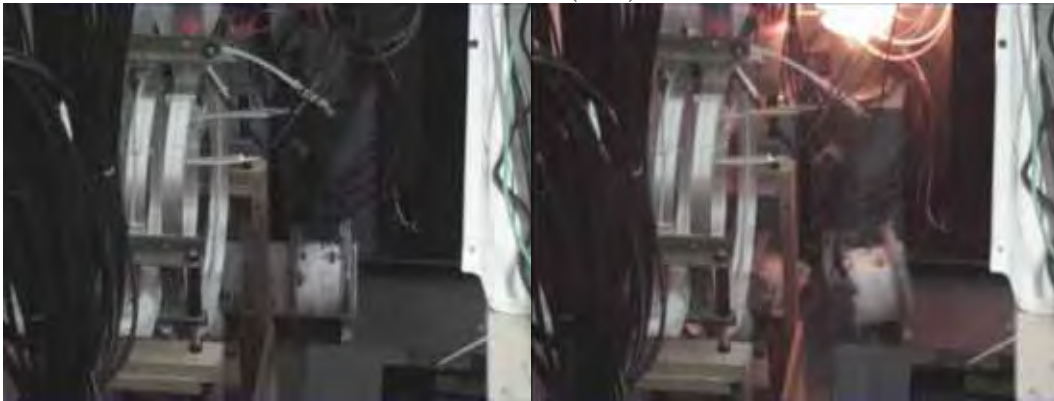
Figure 4.14.1. The price of ringing \theta . Before this shot only the bias and reversal fields (with crowbar) were being fired. (top) At time zero the bias fields are fired followed by the ringing theta at 80 \mu\text{s} and reversal fields at 92 \mu\text{s} .
