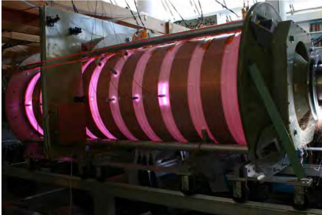
Figure 3.9.7.3. Axial support rods under vacuum loading. The red lines have been added as a reference for comparison. The deflection can be seen (deflection \sim 20\% of diameter, 0.5'' deflection) viewed at an angle likely to indicate only 70% of the total deflection. This figure is intended to emphasize how easy it is to overlook such a seemingly large deflection, not to quantify it, as the rod may have been bent to begin with due to earlier use on a longer experiment or due to original manufacturing deviances. Note that other structures that should be straight show as straight, lowering the probability of a camera lens aberration explanation.
