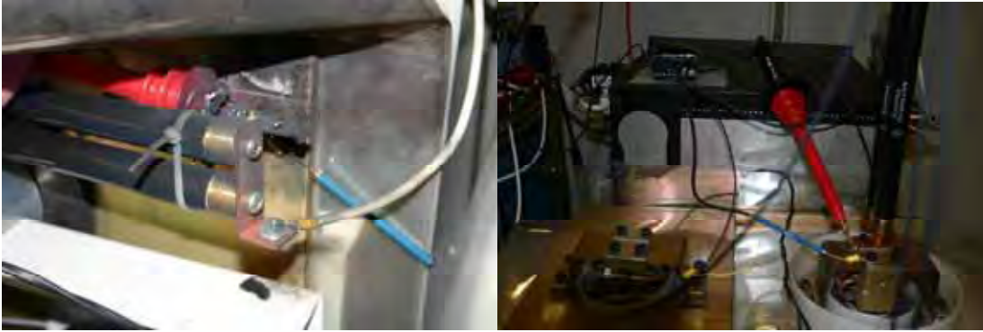
Figure 4.2.1. Commercial high voltage probes can fail. (left) The forward section of a high voltage probe (red) after an explosion occurred. (right) An example of an intact probe connected in a proper manner (so long as the power supply case is grounded). The majority of the rest of the probe ended up as a dust cloud. The probe was placed with its plastic handle too close to a high voltage plate (the plastic was slightly conductive). With the policy of not allowing any non-grounded connections to penetrate the experimental enclosure this was simply a very loud nuisance.
