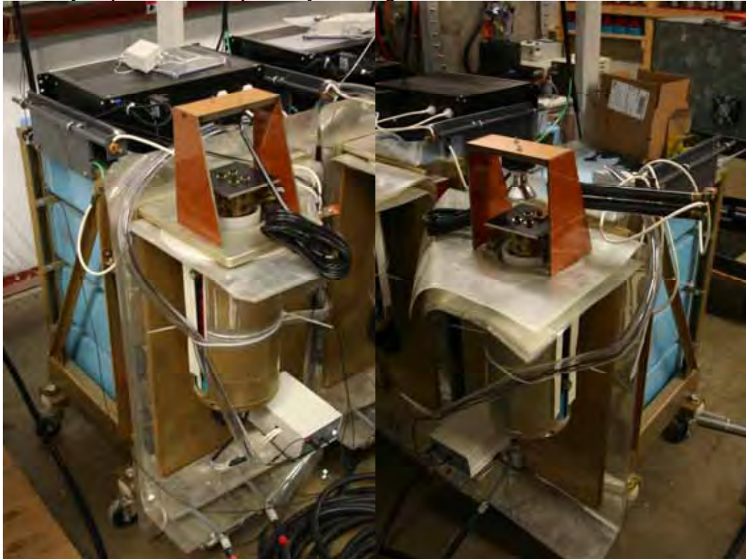
Figure 4.10.1. Bias modules. (left) - polarity. (right) + polarity. These pictures were taken during reconstruction after the latest move. Some parts are missing.
