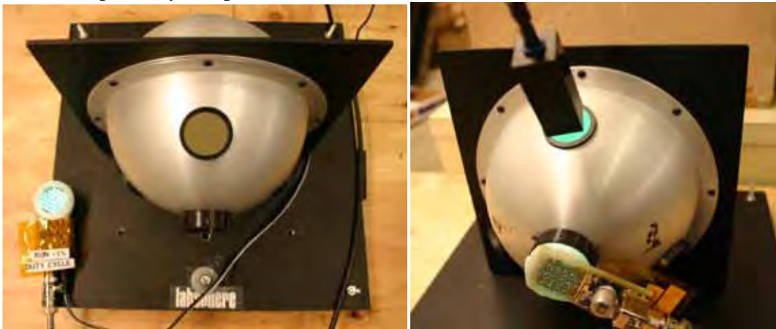
Figure 5.4.3. Integrating sphere and LED light source used for calibrating optical diagnostics response
