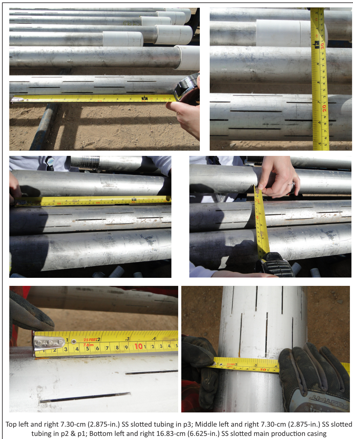
Figure 3-4 Well ER-3-3 Photograph of Slots in the Casing (March 2016)
