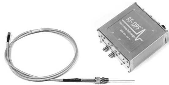
Figure 8. RF measurement system including sensor control unit and measurement probe.
