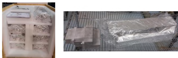
Figure 2. New “inner girders” for the SAGIVU received from ADC. Left: unpacking in the ID lab of NSLS-II. Right: one girder is placed together with a prototype foil stretching mechanism part.
