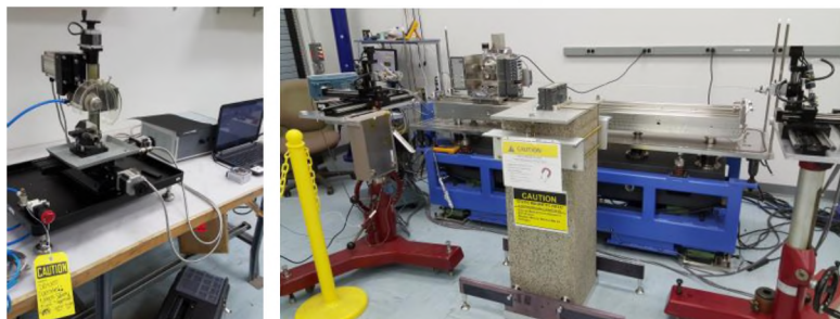
Figure 5. Left: new high-precision computer-controlled diamond disc saw, purchased and customized for shimming of the poles, is ready for validation of its operation by the Safety Group. Right: 1.5 m long magnetic bench is prepared for measurements of SAGIVU magnet girders during their magnetic assembly and shimming.
