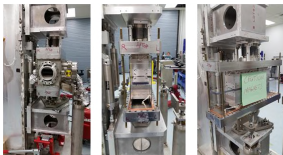
Figure 1. Mechanical carriages of old mini-gap IVU in the ID lab of NSLS-II. Left: vacuum chamber is still present, middle and right: it is disassembled and the “native” inner girders can be seen.
