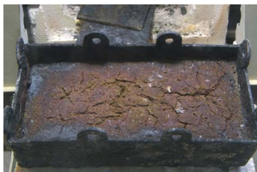
Figure 15. Post-calcination Batch B Vessel and Material Sitting on Furnace Door
