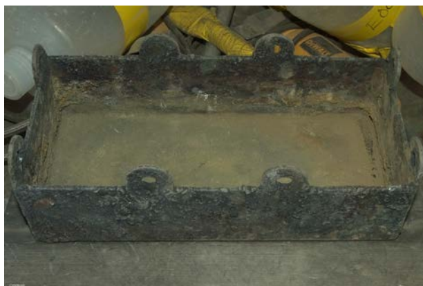
Figure 17. Batch B Calcination Vessel after Material Removal
