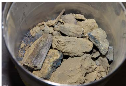
Figure 13. Batch A Stratified Layers in Post-calcination Material
