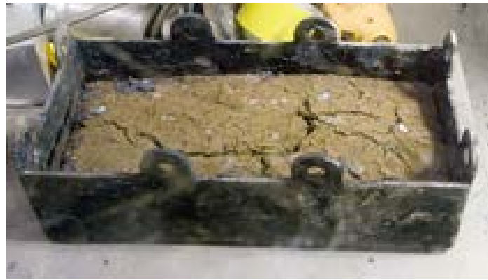
Figure 11. Batch A Material and Vessel after Calcination
