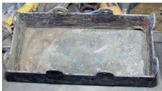
Figure 14. Batch A Calcination Vessel after Material Removal
