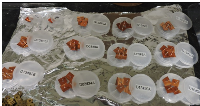
Figure 2: Microclad samples after being bonded to mounting studs with cured epoxy.
