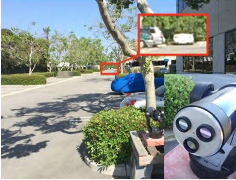
Figure 4. STL parking lot tests. The RGB WFS is approximately 175 meters from the target vehicles. These tests confirmed our ability to get pixel shifts and helped determine how to correlate these shifts to defocus.
