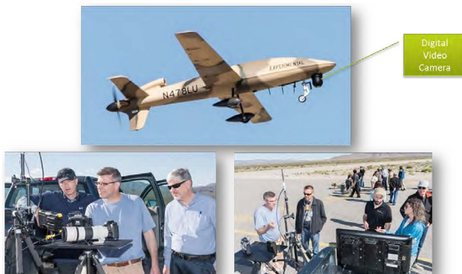
Figure 5. UAS digital video camera and ground monitoring system showing real-time data
