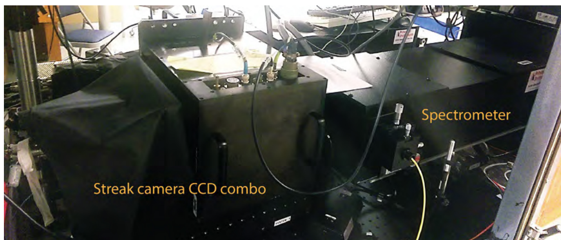
Figure 3. Acton SpectraPro SP-2750 spectrometers coupled to NSTec L-CA-24 optical streak camera
