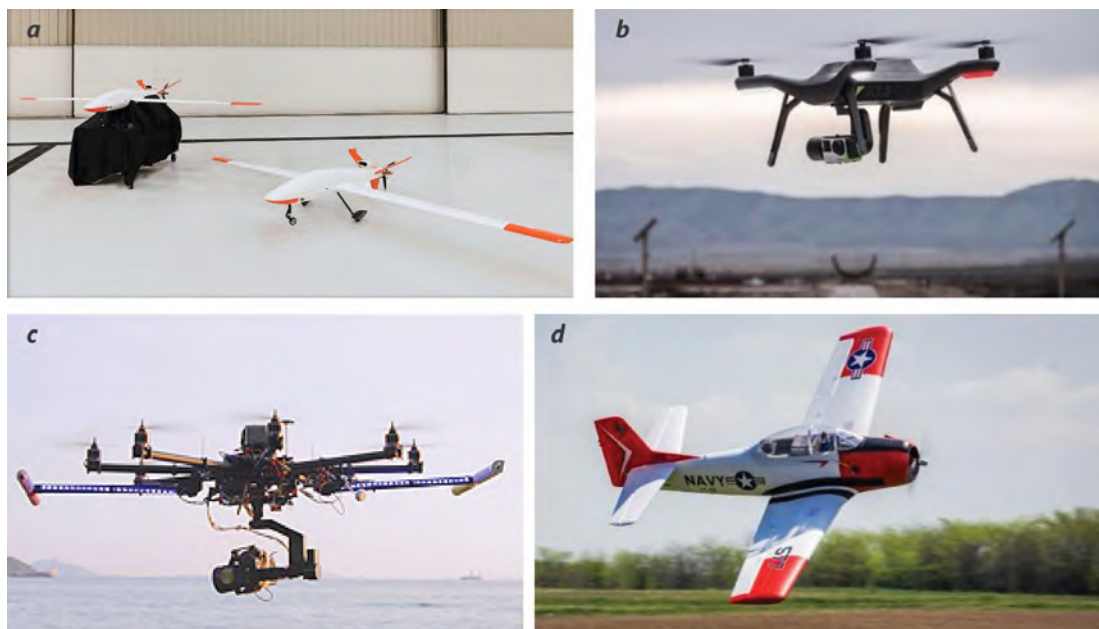
Figure 1. NNSS UAS platforms: (a) Sandstorm fixed wing, heavy payload; (b) 3DR Solo, very small payload; (c) Tarot Octocopter, heavy payload and multi-sensor capable; and (d) T-28 Aircraft, a training aircraft
