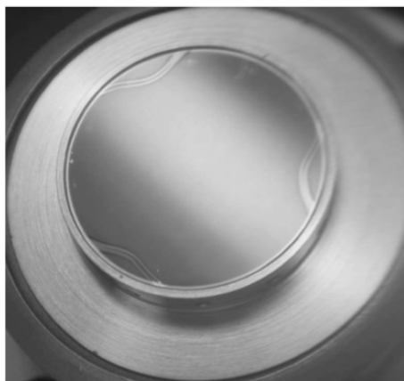
Figure 7. Actual MCP-type PMT with GaN cathode (Siegmund 2008)
