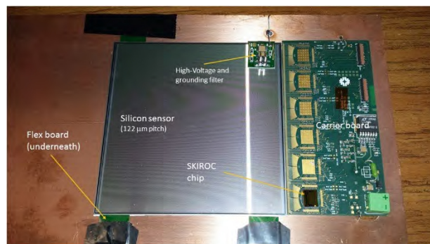
Figure 7. Sensor mounted to readout board for further testing. On the left is the silicon sensor. The microstrips run from left to right, and the sensor is nominally 10 cm on a side. The strips are wire-bonded to the readout board using an automated wire-bonding machine. The photo also shows only one SKIROC chip (the ASIC) mounted for this test. Six will be used on a fully populated board.
