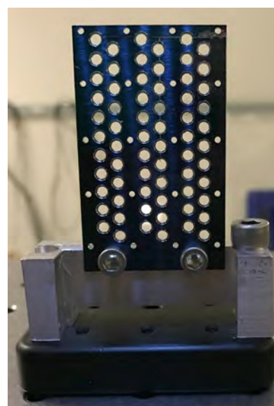
Figure 6. Next-generation target holder with nanowire arrays mounted in holes to isolate the laser damage
