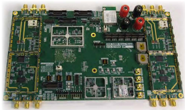
Advanced SDR test platform developed for an FY 2013 SDRD project (Fay 2014)
