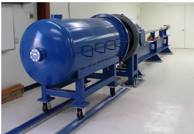
Figure 1. The new propellant launcher, installed in Building 229 at STL, is capable of launching projectiles at 0.5 to 2.5 km/s, which expands the velocity range considerably for shock compression experiments
