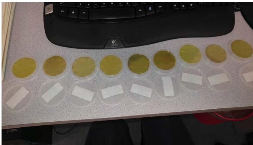
Figure 9. Nine unique wafers grown using the two parameters of InGaN absorption thicknesses (100, 150, 200 nm) and AlN surface caps (0, 5, 10 nm)
