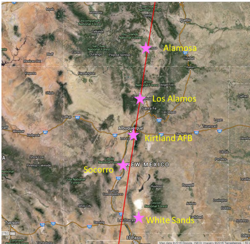
Figure 3. Geomagnetic meridian geometry of the Los Alamos, New Mexico experiments. AFRL ionosonde stations at Kirtland AFB, the Very Large Array, the Long Wavelength Array, and White Sands Missile Range fall on or near the Los Alamos geomagnetic meridian. Also shown is a possible site for portable monitoring systems near Alamosa, Colorado. Image courtesy of AFRL.
