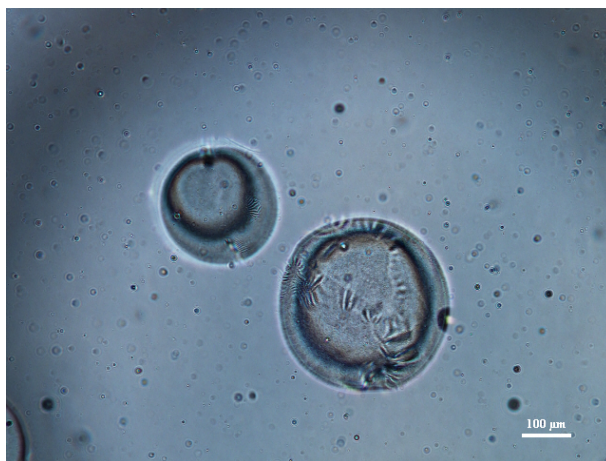
Figure 3.2. Imperfections in capsule shell surface due to high viscosity of TE-2000 and voids.
