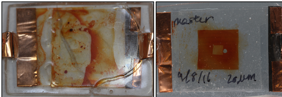
Figure 3.14. Cracking within flexible EPD cell resin encasing, as a result of long dithiol chain length (left) in comparison to short chain length dithiol resin (right).
