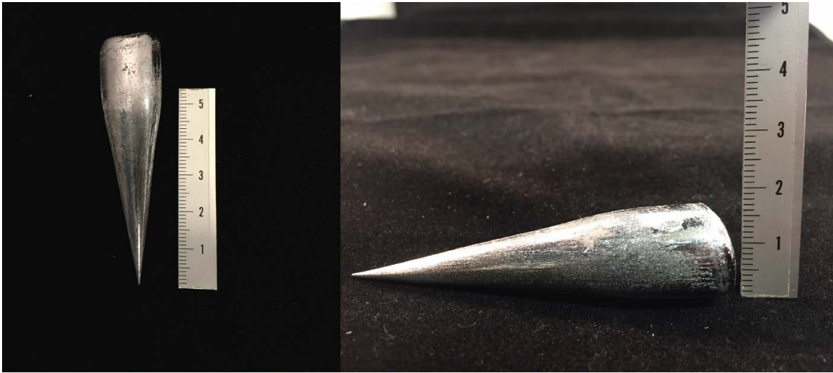
Figure 2: Ingots of \text{BiI}_3 grown through the Bridgman method with superheat gradient modifications.
