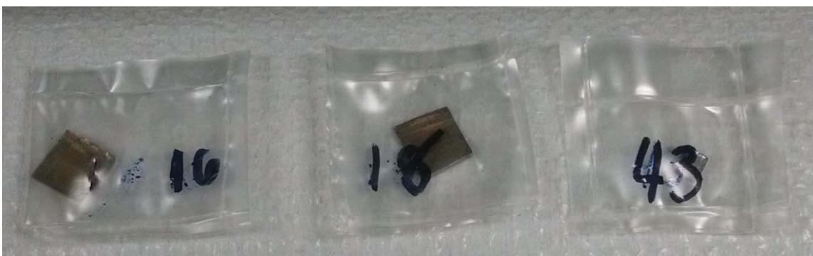
Figure 36 - Samples 16, 18, and 43 still sealed in polyethylene after irradiation at 0.1 kW
