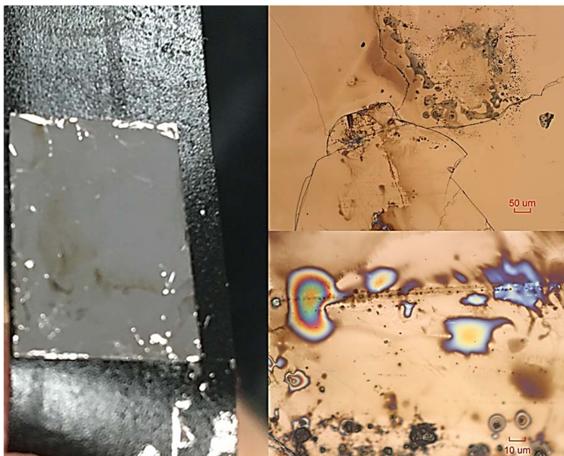
Figure 27. The cleaved Bi surface where extended defects were located. Two different reactions were identified.
