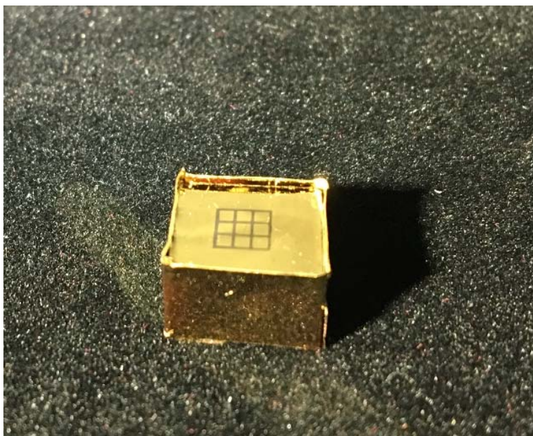
Figure 19. Bil 3 crystal with a 3 x 3 pixel electrode grid following Au electrode deposition.
