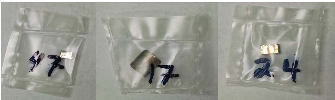
Figure 37 - Samples 17, 24, and 47 still sealed in polyethylene after irradiation at 1 kW
