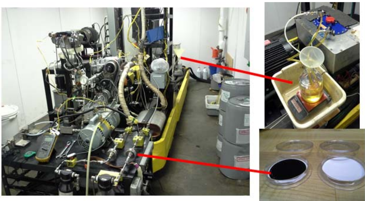
Figure 11 A soot sampling cart was developed and used to collect raw particulate matter for elemental testing. Fuel consumption was estimated using a scale as depicted on the right.
