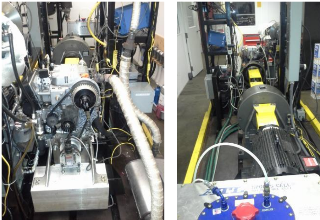
Figure 6 Fore and aft views of engine test cell rig [2].
