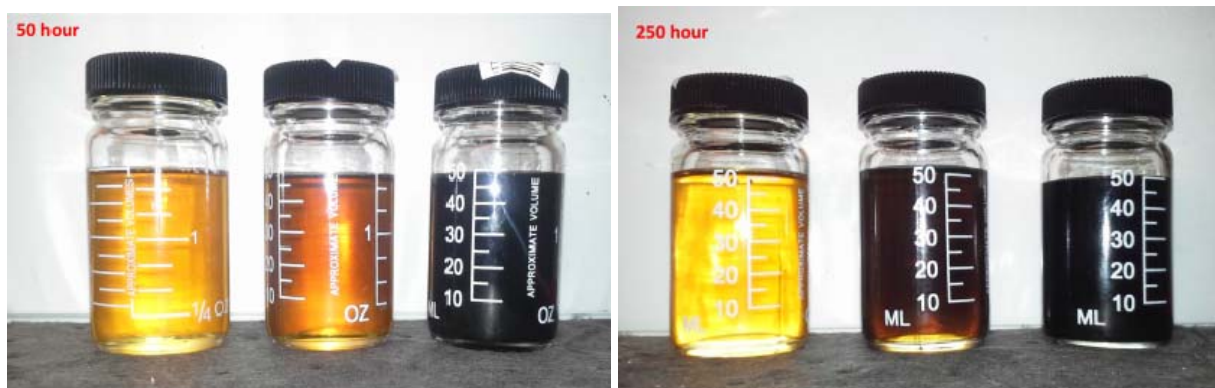
Figure 43 Oil samples at 50 and 250 hours. New oil is on the left of each photo. The valve train sample is in the center, and power cylinder lubricant sample on the right [2].
