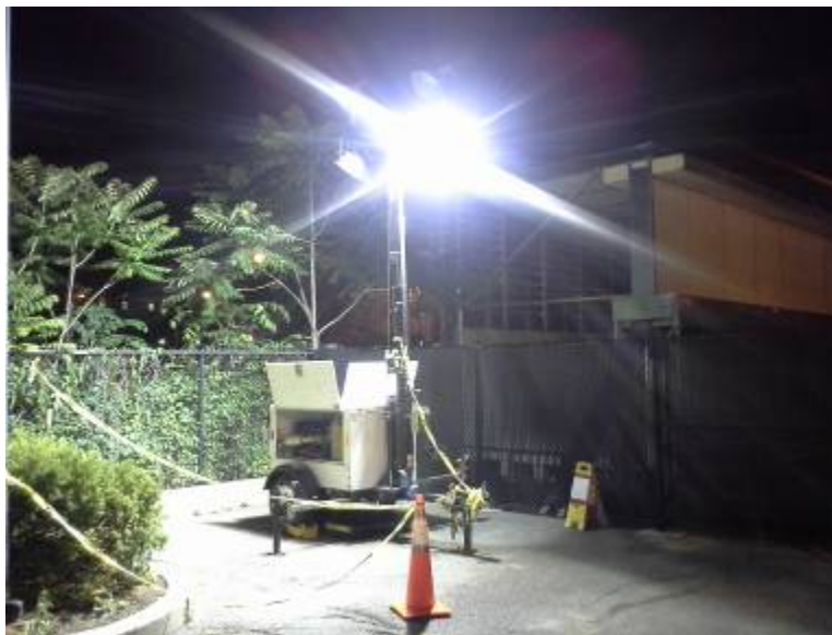
Figure 12 A full scale field test was conducted over a period of 4 weeks. The engine was operated for 250 hours to provide data on oil aging in each engine subsystem. Samples were sent to an independent lab for analysis. Results are expected next quarter.
