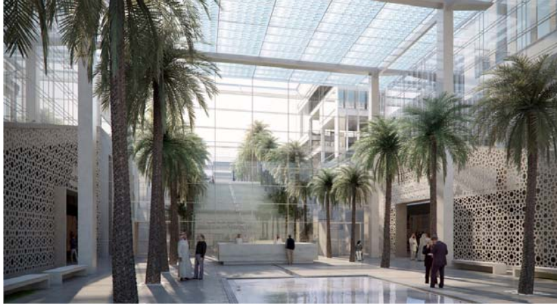
Figure 120. SKMC General Hospital Lobby with transparent ICSF roof modules that bathe the interior space with cool diffuse daylight and allow for a clear view to the sky while removing solar heat gain and glare from the space.
