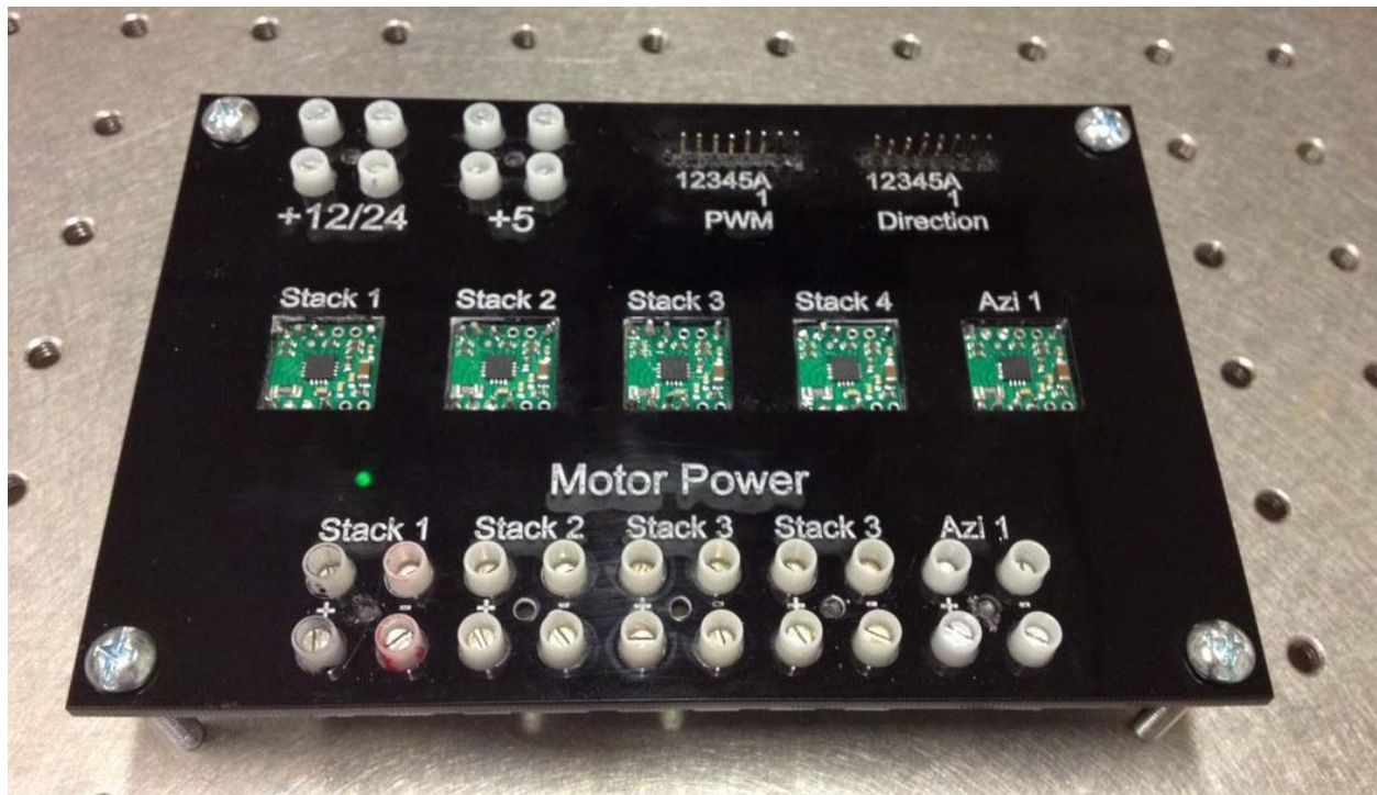
Figure 112: Fabricated Motor Control Board to House Motor Drivers.
