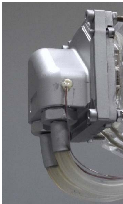
Figure 27. ICSF Generation 7 prototype, deployed at CASE studio, Manhattan, NY. Improvements include an optimized optical design, and simplified mechanical design for manufacture, assembly, and operational robustness. Coolant-fed heat sink revised. The Fresnel-Kohler primary and secondary optics provide uniform flux on the CPV cell while easing the tracking accuracy requirements.
