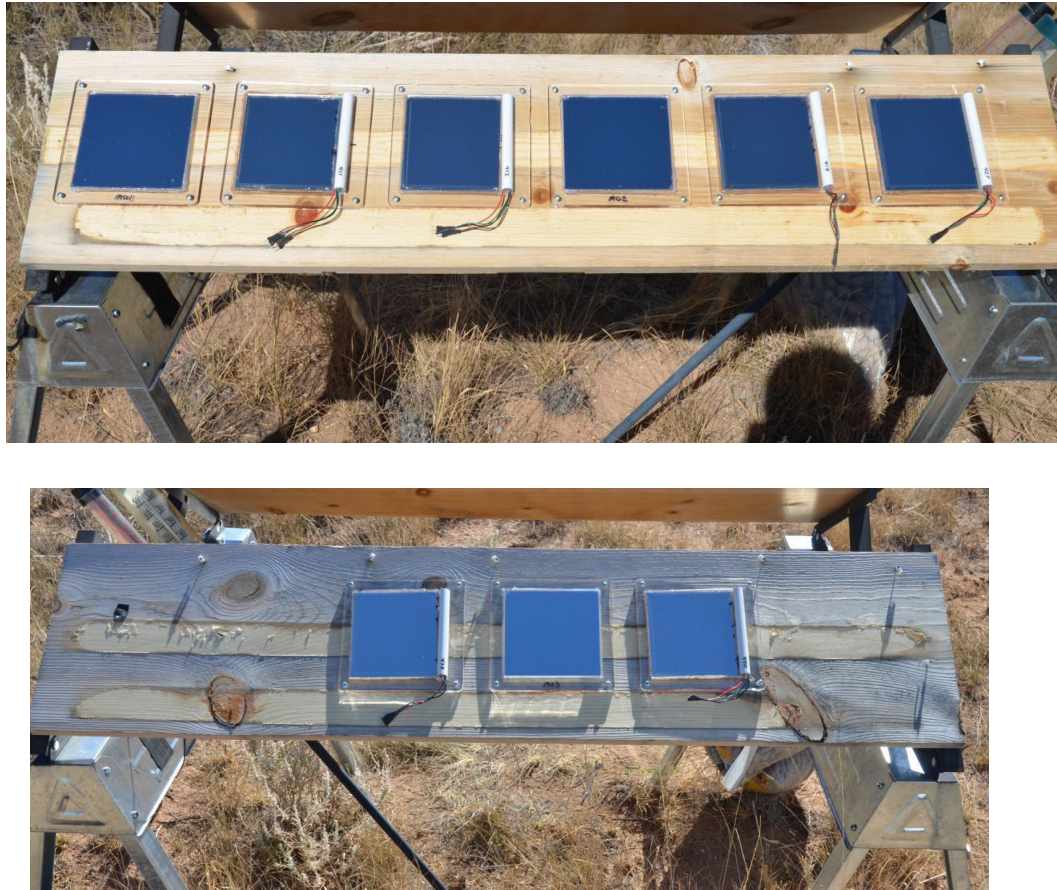
Figure 22 - Photograph of the six EDS (top row) and three control (non-EDS) mirrors in place for long-term testing at the SNL solar field
