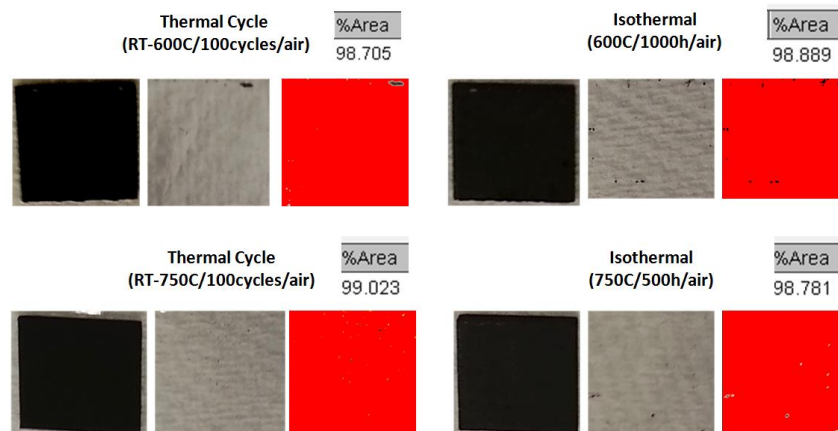
Fig. 32. Adhesion evaluation for CFM(PT)/CuCr 2 O 4 (DB) sample after thermal tests. In each thermal test, The left is the sample image after removing tapes, the middle is the image of the detached tape, and the right is ImageJ-processed image which yields the retained area percentage.
