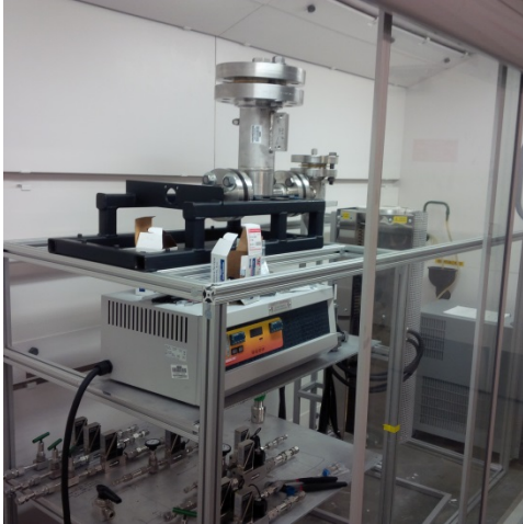
High pressure pyrolysis reactor and GC/Mass spectrometer used for analysis.
