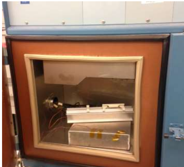
Figure 178: Clip, rail assembly in thermal chamber
