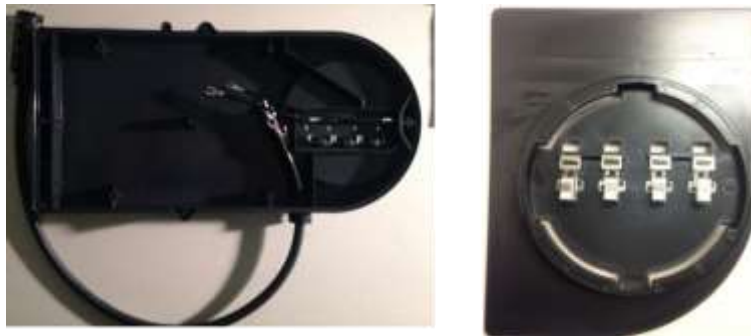
Figure 176: Micro-inverter enclosure and panel connector
