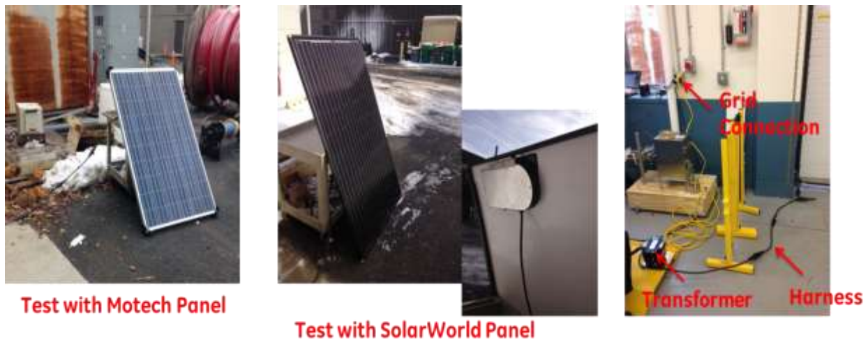
Figure 186: Outdoor test of ACPV panels
