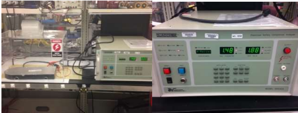
Figure 145: Ground leakage current test setup and test result at 1480VAC
