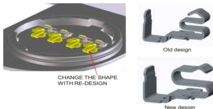
Figure 174: Modifications to spring contacts
