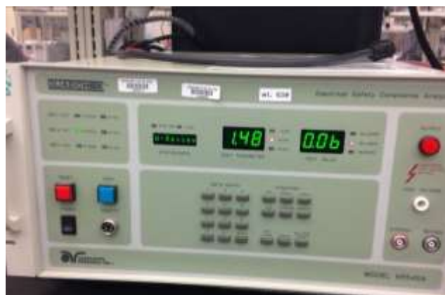
Figure 147: Dielectric test after modifying resistors - unit passes
