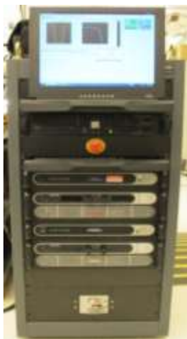
Figure 66: TerraSAS PV Emulator with Two Channels
