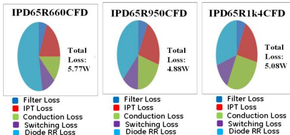
Figure 110: Inverter loss breakdown using different switches
