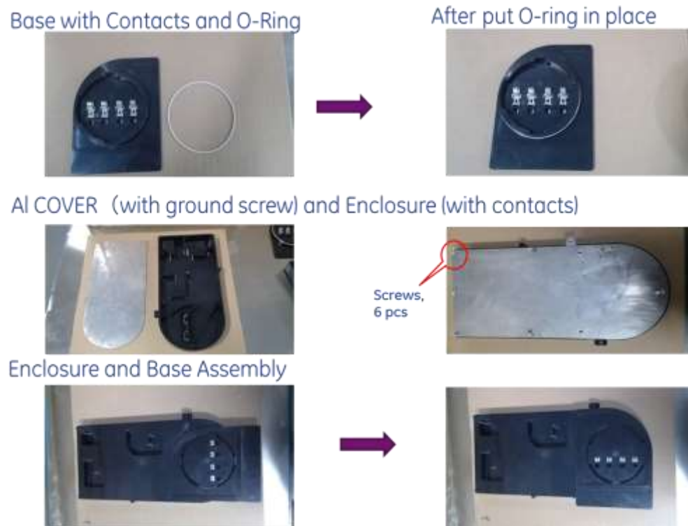
Figure 131: Pocketed inverter boxes and panel connector from Amphenol
