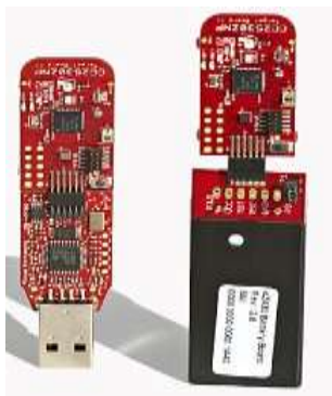
Figure 90: Zigbee System-On-Chip Kits (TI CC2530)
