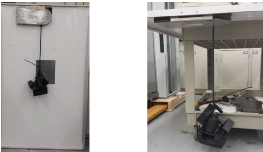
Figure 171: Mechanical loading of SolarWorld ACPV panel
