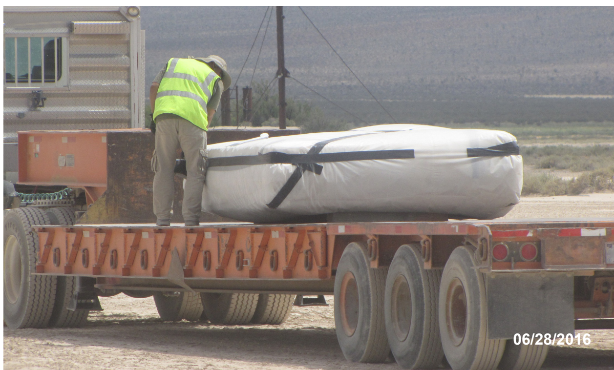
Figure 2-11 Concrete Slab Wrapped and Loaded for Transport
