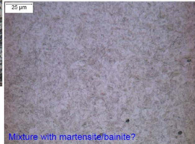
Figure 17. Microstructures from an alloy 2 keel block warrant further characterization, as do the microstructures from most of the alloys studied [2% Nital 500x]
