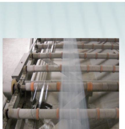
On-line produced IEL on <1.8mm glass using long slots
