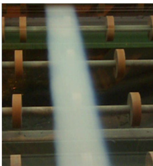
Figure 3 Glass substrate with IEL produced in PPG/Vitro on-line process.
