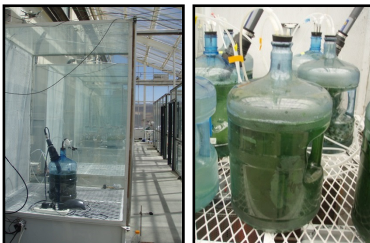
Figure 5. Incubation vessels instrumented with gas lines for air delivery and analyses as well as water quality (e.g. dissolved oxygen, pH) sensors
