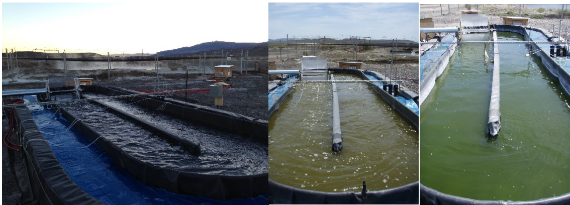
Figure 7. Pilot-scale raceway (with inner production raceway and outer temperature control raceway) that was built and operated at Olam Spices and Vegetable Ingredients, Inc. near Fernley, NV. The geothermal source water was contained in the cooling pond in the fenced area behind the raceway. The two images on the right show two sets of experiments/ manipulations with different microalgal consortia at different temperatures.
