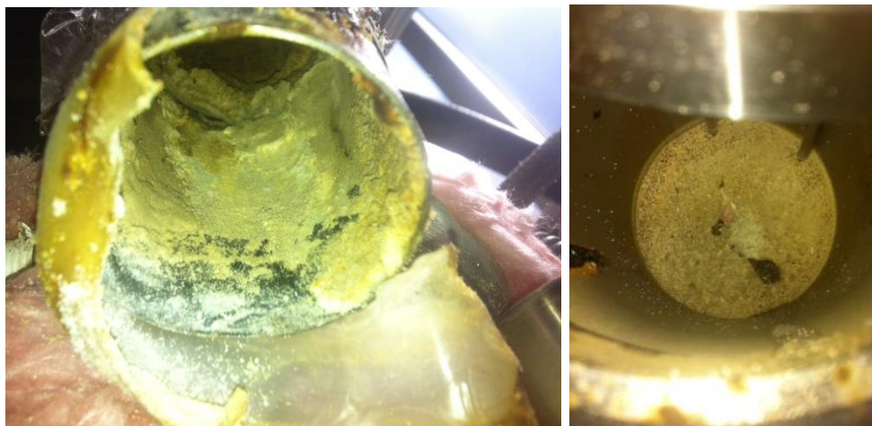
Figure 45. Pellet sample adhered to piping above the desorber and covers the vent to allow recirculation of the gases inside the desorber.
