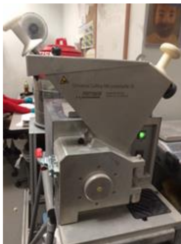
Figure 7. The large mill used to pulverize the AFA sorbent to micron size particles.
