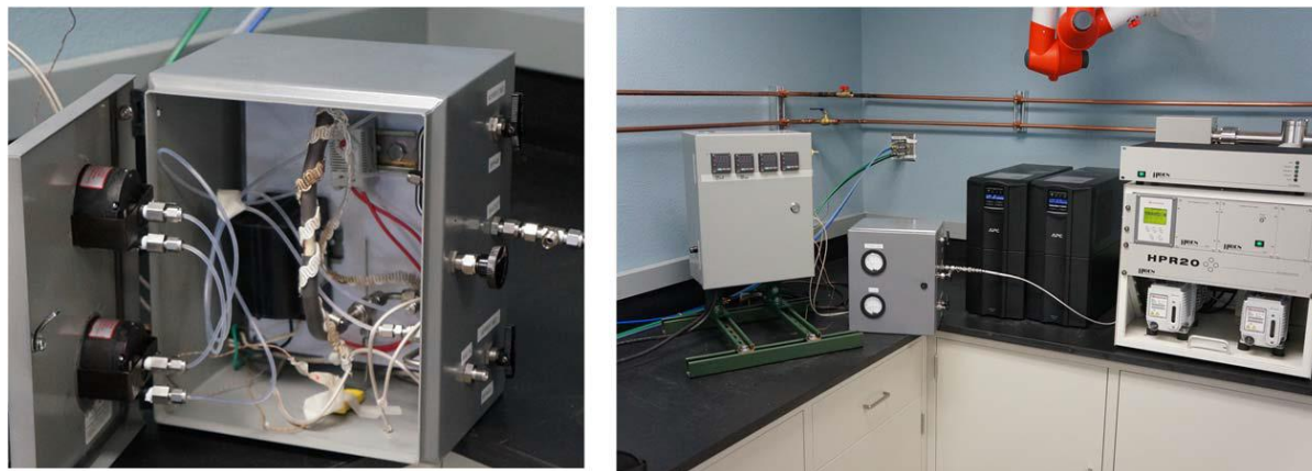
Figure 5. Mass spectrometer-fixed bed (right); detail of heated fixed bed enclosure (left).
