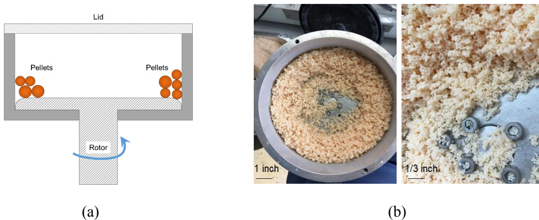
Figure 9. (a) Illustration of the homemade spheronizer, (b) Spheronized AFA sorbent pellets in the spheronizer.
