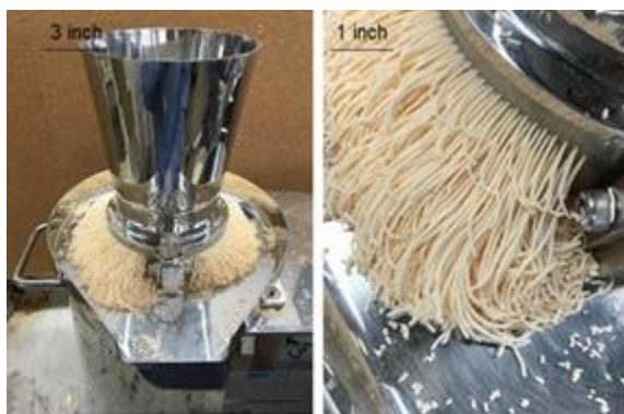
Figure 8. Commercial basket extruder and the extrudate (AFA sorbent + binder).
