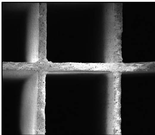
Figure 7, ZnO Coated On Cordierite Monolith Structure.
