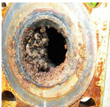
Figure 7 Ash and tar in gasifier
