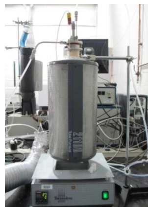
Figure 1: Schematic of experimental setup for the matrix solubility measurement. A photograph of the test-up is also shown.
