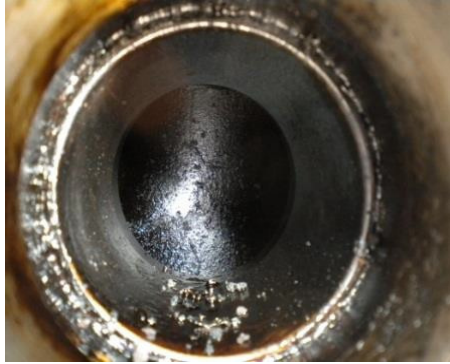
Figure 8 Tar accumulations in piping
