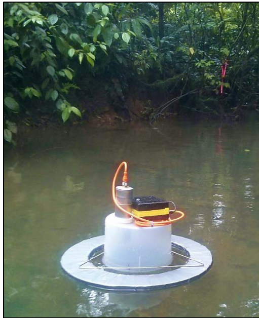
Figure 2. Floating chamber deployed in the Arboleda stream for all drifting measurements and for the comparison between static and drifting modes conducted on 16 August 2014. The area of stream coverage by the chamber alone was 0.041 \text{ m}^2 , and the chamber volume = 5.6 L. The gray ring around the chamber is a Styrofoam piece installed \sim 5 \text{ cm} from the outer wall of the chamber for floatation.
