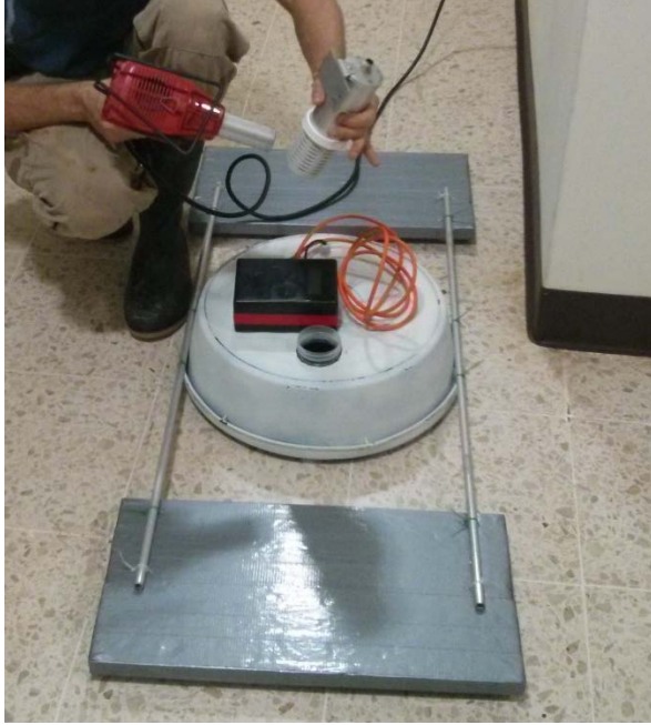
Figure 1. Floating chamber used for measurements in static mode. The area of stream coverage by the chamber alone was 0.126 \text{ m}^2 , and the chamber volume was 10.9 L. The gray plates are Styrofoam pieces installed \sim 10 \text{ cm} from the outer wall of the chamber for floatation.
