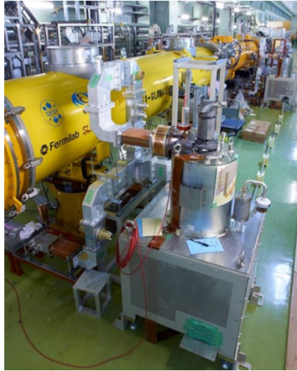
(a) DRFS klystron in the S1-Global experiment
