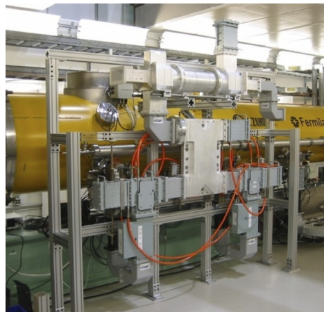
(a) A two-feed unit of PDS1, incorporating a VTO and H-hybrid, installed on a cryomodule at NML.
