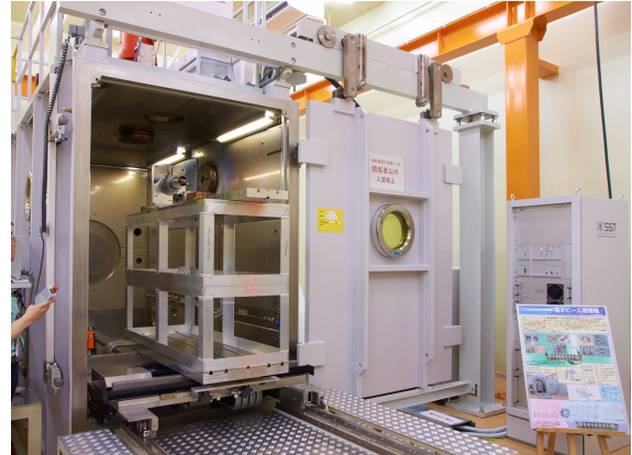
Figure 2.2 The Cavity Fabrication Facility at KEK showing the electron-beam-welding setup.
