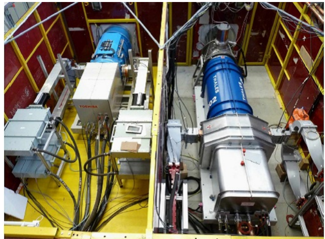
Figure 2.53 Horizontally mounted MBKs; (left) Toshiba E3736, (right) ThalesTH1801.
