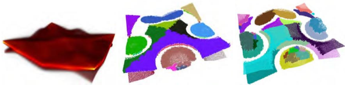
Figure 12: On the left, a volume rendering of a hixel data set generated by sampling images 3200 samples of a Poisson distribution and 9600 samples from a normal distribution. There are 512 \times 512 hixels in this data set, each with 128 bins. The shortest axis in the images corresponds to histogram bins, thus a spatially higher location along that axis indicates a higher function value. Color and opacity are used to illustrate the density of samples. Thus the lower, right corner of shows a hixel with 2 distinct probable function values; the smaller function value is less probable than the larger. The center image shows basins of minima and the right image shows basins of maxima for this data set. By computing basins on sheets we are able to identify prominent features associated with each process in the mixture model.
